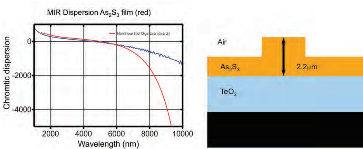
Figure 1 (a) Calculated dispersion of  $As_2S_3$  waveguides in the mid-infrared and (b) schematic of a  $As_2S_3$  waveguide that employs a  $TeO_2$  substrate.
