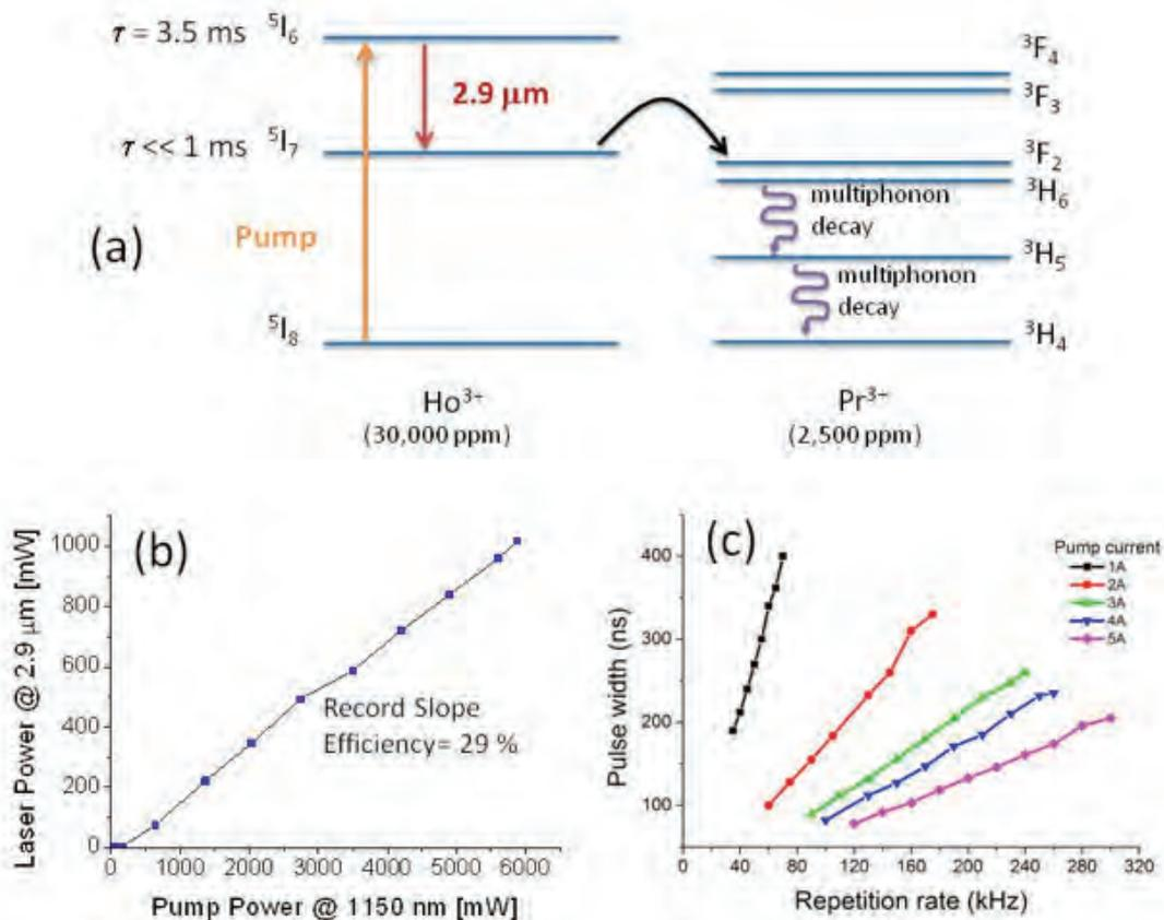
Figure 2 (a) Schematic diagram of the  $\text{Ho}^{3+}$ ,  $\text{Pr}^{3+}$ -co-doped systems showing the pump, laser and energy transfer processes, (b) Output power vs input pump power of the tunable  $\text{Ho}^{3+}$ ,  $\text{Pr}^{3+}$ -co-doped fibre laser at tuning range centre and (c) pulsewidths from a Q-switched  $\text{Ho}^{3+}$ ,  $\text{Pr}^{3+}$ -co-doped fibre laser as a function of repetition rate of the acousto-optic modulator.
