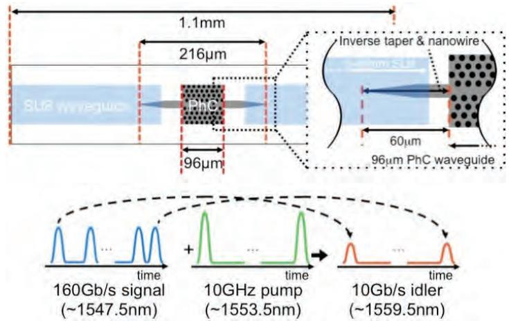
**Fig 2:** Schematic of the engineered photonic crystal waveguide chip and four-wave mixing based de-multiplexing scheme. Inverse tapers mediate coupling from fibres to nanowire waveguides, which are butt-coupled to the photonic crystal waveguide. On chip, a 160Gb/s signal is mixed with a 10GHz optical clock used to pump the four-wave mixing interaction. The idler product of the nonlinear mixing is a 10Gb/s tributary channel of the 160Gb/s data stream.
