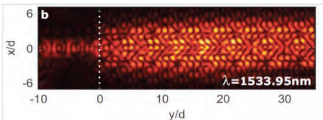
**Fig 7: Local intensity versus position in a silicon photonic crystal with a waveguide. The vertical line indicates the boundary between the incident medium on the left where the light travels at a speed close to that in bulk silicon, and the slow medium on the right where the light travels at a fraction of the speed of light.**
