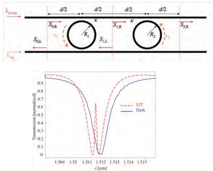
**Fig 5: Top: Schematic of the coupled microring resonators structure. Bottom: Probe transmission spectra without pump (dashed curve) and with pump (solid curve).**
