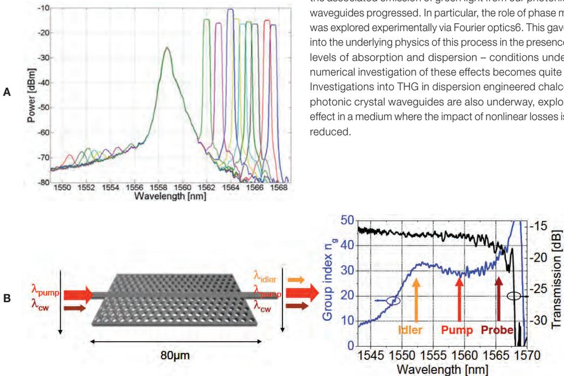
**Fig 1:** a) FWM spectra of the slow PhC waveguide for different probe wavelengths when launching a constant coupled probe power of 400 $\mu$ W, and a coupled peak pump power of 1W. b) Schematic partially degenerate FWM in the probed planar PhC waveguide. The pulsed pump and CW probe mix to create an idler wave. (right) Spectral variation of the group index for the dispersion engineered PhC waveguide with the wavelength of the probe, pump and idler highlighted.
