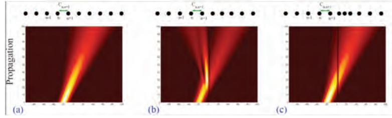
**Fig 4: Top row: schematic of coupled resonator optical waveguides with (a) homogeneous arrangement, (b) modulated coupling, and (c) special reflectionless modulation. Bottom row: pulse propagation dynamics.**
