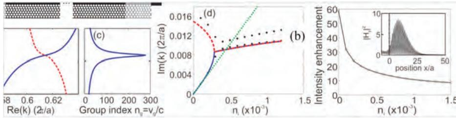
**Fig 6: (a) Schematic of photonic crystal waveguide with (i) regular and (ii) slow group velocity regimes. (b) Maximum intensity enhancement vs. loss parameter  $n_i$ . Inset shows normalised magnetic field along the waveguide axis for  $n_i = 1.5 \times 10^{-3}$ , where the interface between fast and slow sections lies at  $x = 0$ .**
