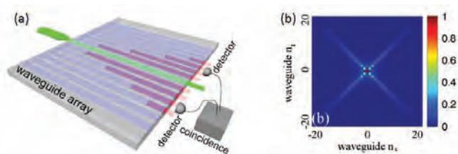
**Fig. 3. (a) Schematic of a quadratic waveguide array: The pump beam generates photon pairs that couple to the neighbouring waveguides where quantum walks take place. (b) An example of photon-pair correlations (bunching) in real space (waveguide numbers) for a pump coupled only to the central waveguide  $n=0$  with zero single-waveguide degenerate phase mismatch.**
