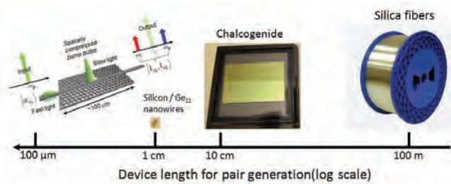
**Fig. 1. Development of miniaturisation of photonic devices for photon-pair generation.**
