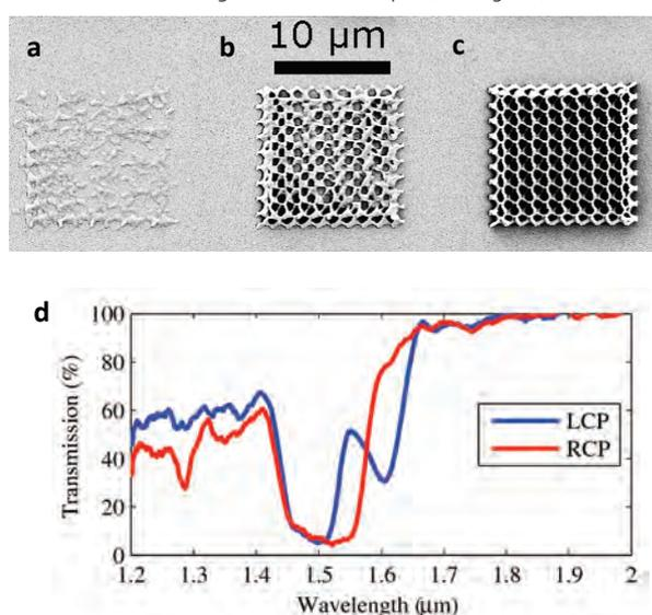
**Fig. 4. Fabrication of 3 polymer chiral Gyroid srs-networks of unit cell size  $1.2\ \mu\text{m}$ . a) No galvo-dithering is used - the structure is mechanically weak. b) A small dithering is used, with small improvement in structural integrity. c) The correct amount of dithering is used greatly improving structural integrity and optical quality. d) Experimentally measured transmission spectra of the improved Gyroid srs-network, for left (blue) and right (red) circularly polarised light.**
