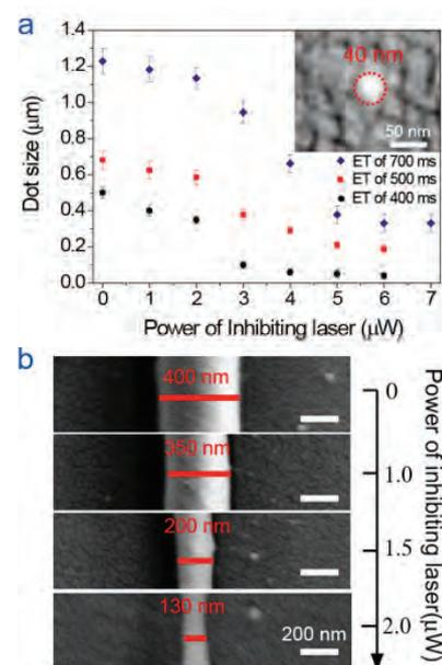
**Fig. 1** (a) Dot sizes are plotted as a function of the power of the inhibition laser and SEM image of the dot fabricated with the exposure of the initiating laser and the inhibiting laser beams of the power levels of 200 nW and 6 μW, respectively, at the exposure time of 400 ms. (b) SEM images of lines fabricated with different power levels of the inhibiting laser, at a fixed scanning speed of 3 μm/s, and under the irradiation of initiating laser beam of 200 nW.
