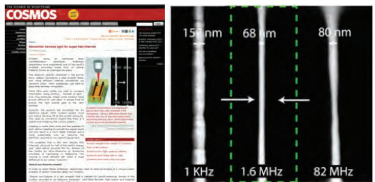
**Fig. 3 (a) COSMOS magazine story covering the realisation of nanowire in nonlinear materials [7]. (b) SEM image of nanowires fabricated under different laser repetition rates showing an optimal resolution of 68 nm at a repetition rate of 1.6 MHz.**
