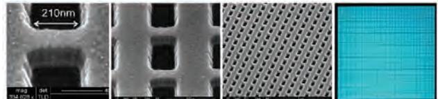
**Fig. 4:** Fishnet metamaterials fabricated using lift-off process – the dielectric (MgF) is clearly visible between the upper and lower gold layers. The fishnets cover a 4x4mm square which was fabricated overnight using the e-beam lithography tool at RMIT.
