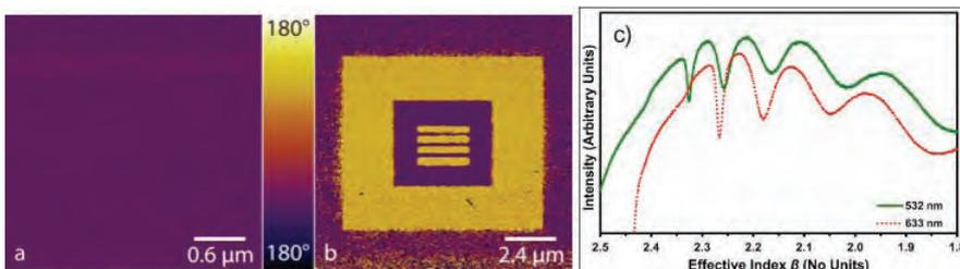
**Fig. 3:** Analysis of SBN thin film from a) PFM showing as grown film is single domain; b) PFM after poling with an AFM tip showing nano-scale patterning of domains is possible; c) prism coupling results enabling measurement of thickness and refractive index.
