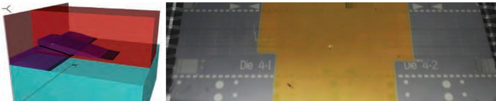
**Fig 2. LHS, a schematic of a taper coupler used to convert a mode from a polymer waveguide matched to UHNA-3 fibre to a highly nonlinear  $As_2S_3$  rib waveguide; RHS a photograph of the fabricated device showing the tapered chalcogenide layer (yellow) connected to SU8 input waveguides.**
