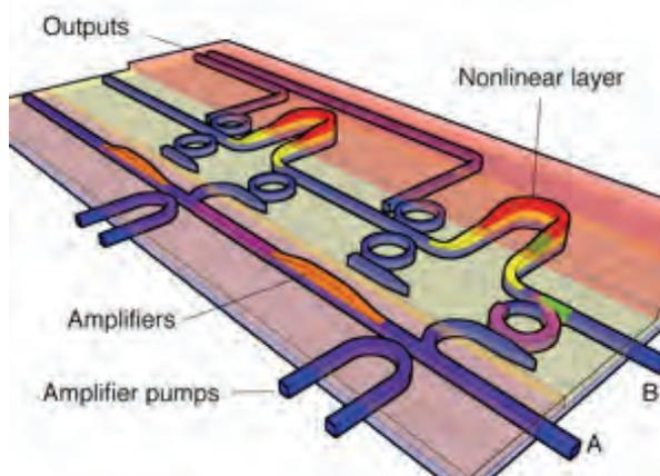
**Fig. 1.** The hybrid circuit concept being pursued by CUDOS involves vertically stacked layers of materials offering different functionalities coupled by vertical tapers. This example is creates a multi-channel all-optical demux.
