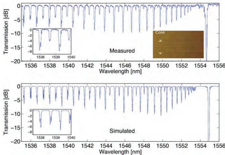
**Fig. 1.:** Measured and calculated cladding-mode spectra for a laser written fibre Bragg grating. Insets show an image of the grating and the polarisation splitting predicted by the vector theory.
