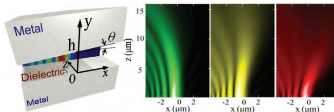
**Figure 2:** (left) Wedged metal-dielectric-metal structure for manipulating Airy plasmon with one metal plate tilted by an angle  $\theta$ . (right) Numerically calculated field distributions of three plasmonic Airy beams at wavelengths of 0.6, 1 and 1.4 μm (in false colours) and  $\theta = 0.458^\circ$ .
