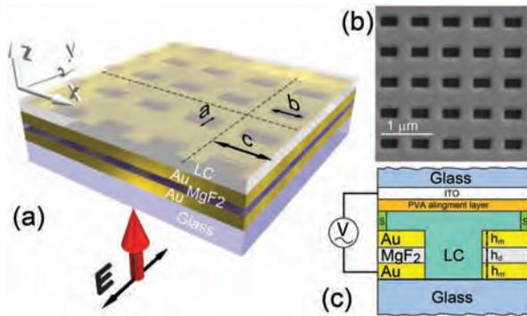
**Figure 1:** (a) Schematic of the fabricated LC infiltrated fishnet metamaterial. (b) Scanning electron microscope image (top view) of the fabricated structure. (c) Side view of the LC cell: DL is a dielectric layer, S - 100 μm thick plastic spacers. Parameters for the fabricated Au-MgF<sub>2</sub>-Au fishnet are  $h_d = h_m = 50$  nm,  $a = 190$  nm,  $b = 350$  nm, and  $c = 600$  nm.
