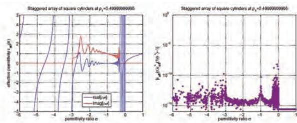
**Figure 4.** Left: the effective relative permittivity of a staggered array of square cylinders at  $p_1 = 0.4999999995$ . The curves are supported by 2006 adaptively spaced data points. Right: the absolute difference between the left- and right-hand side of (16).
