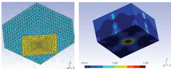
Figure 1: Chequerboard grating: 3D FEM unit cell mesh and contour plot of field intensity.
