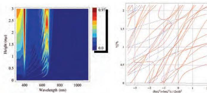
Figure 2: Contour plot of the absorptance of the nanowire array as a function of the wavelength and the wire length, and Bloch mode dispersion curves of a lossless cylinder array.
