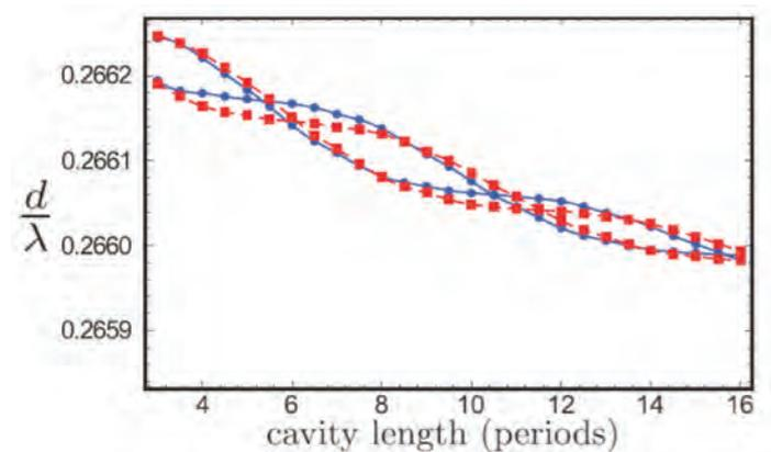
agreement and intuitive insight. For example, when the edges of the light region are graded then the modal frequencies never intersect as the cavity length is altered. Cavities with two high-Q modes which are spectrally separated by a predictable, and easily designed, frequency may have applications in quantum optics.
