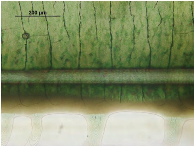
**Fig. 5: Opal-covered tapered optical fibre. The bandgap direction is radial from the fibre axis.**
