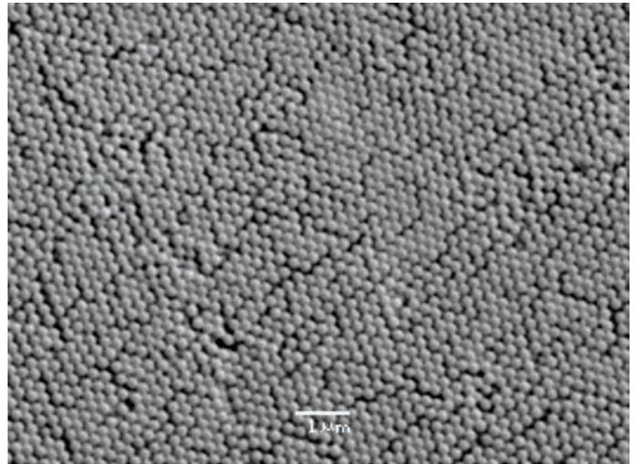
**Fig. 7: Metallized silica spheres assembled to form an opal.**
