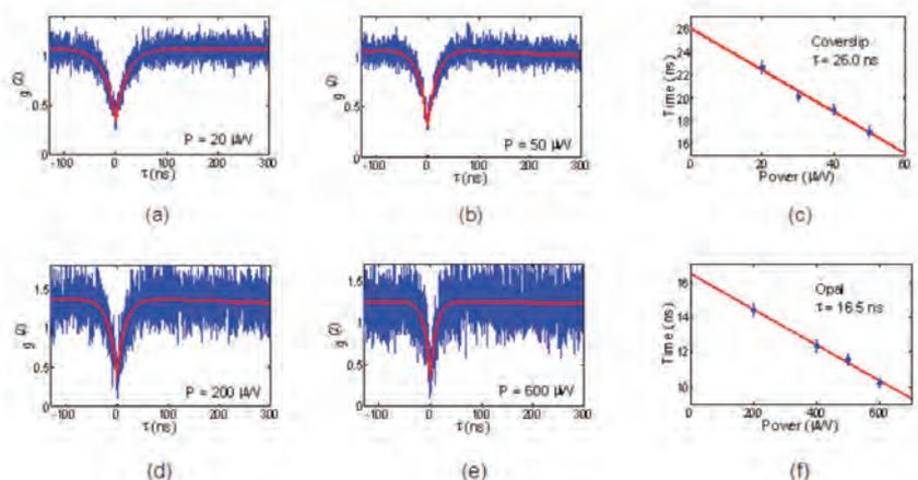
**Fig 1: Averaged lifetime measurements for nano diamonds on flat coverslip and on opal showing typical second order correlation measurements.**
