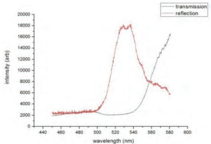
**Fig. 8: Transmission and reflection spectra of metallized opal. Bandgap occurs at 530 nm, which is red shifted by the presence of silver coating on silica spheres.**
