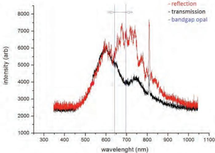
**Fig. 6: Transmission and reflection spectra for light propagating along the opal-coated tapered fibre. The corresponding bandgap of the opal (measured perpendicular to the opal surface) is shown in grey. The spikes in the spectra due to the white light source at 808 nm are attributed to the pump laser.**
