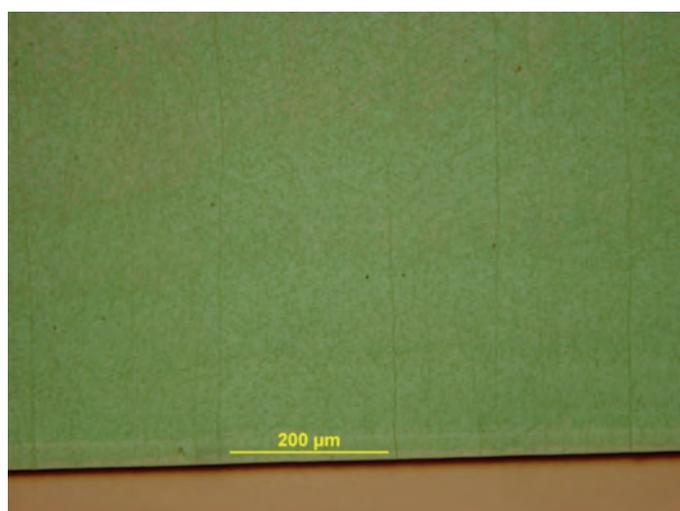
**Fig 4: Optical micrograph of opal showing parallel cracks with wide spacing.**
