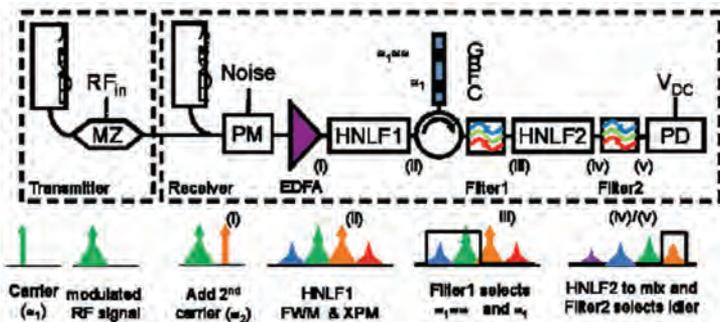
Fig 5: System configuration of the recently demonstrated 'remoted' all-optical IFM [6].
