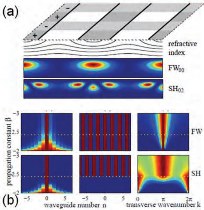
Fig 2: (a) Sketch of the periodically poled lithium niobate sample depicting the refractive index profile and the intensity distribution of the FW and SH modes. (b) Absolute values of the mode amplitudes (left); phases distribution (middle) [blue corresponds to 0 and red to  $\pi$ ]; and absolute values of the spatial Fourier spectra (right).
