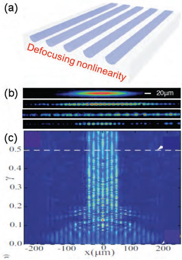
**Fig 1: (a) Sketch of the waveguide arrays. (b) Input beam profile; linear diffraction at the output; nonlinear defocusing at low nonlinearity (time); and beam localization at high nonlinearity. Beam power, 1 mW. (c) Dependence of the output intensity profile on the nonlinearity  $\gamma$ . The beam spreading is arrested at a critical nonlinearity,  $\gamma \approx 0.15$ .**
