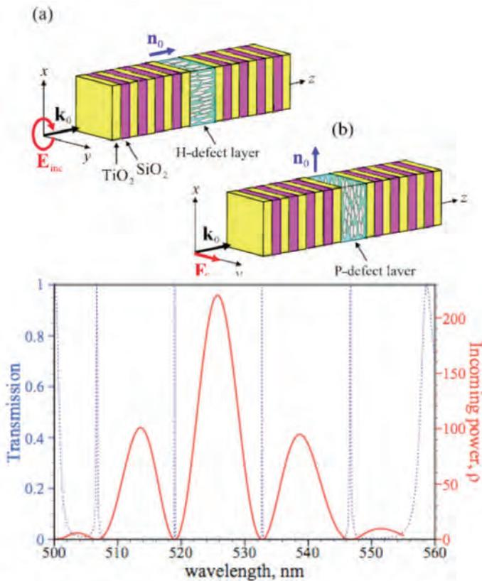
Fig 4: light induced reorientational effects in planar nematic liquid crystals cell embedded into a one-dimensional photonic crystal.
