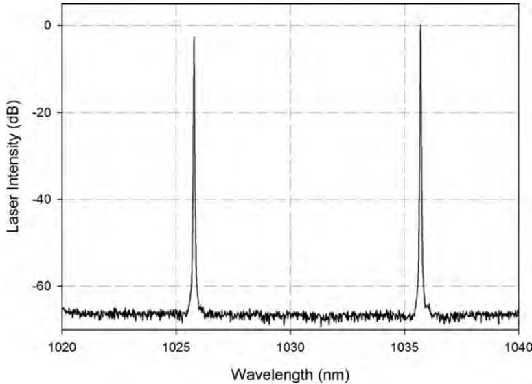
**Fig 2: Dual wavelength laser fabricated in Yb-doped phosphate glass using a phase modulated sampled waveguide Bragg grating.**
