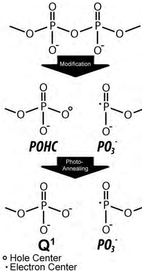
**Fig 4: Colour centre formation/removal in phosphate glass under kHz rep rates. Phosphorous-oxygen hole centres (POHCs) and  $PO_3^-$  ions form as a result of P-O bonds being broken during the modification process, and the subsequent removal of POHCs give rise to the increased proportion of  $Q^1$  P-tetrahedra.**
