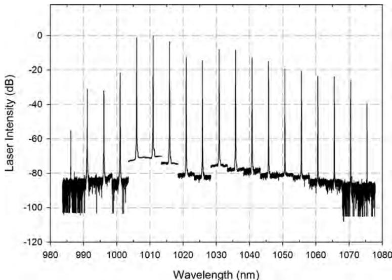
**Fig 3: Single wavelength waveguide lasers operating from 985 nm up to 1075 nm.**
