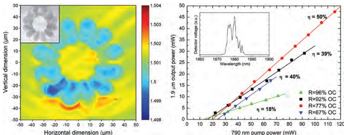
**Fig 5:** Caption: (Left) Absolute refractive index profile at 637 nm of a waveguide consisting of 24 partially overlapping cylinders fabricated at 1000 mm/min. Inset shows the corresponding optical microscope image. (Right) Measured slope efficiency for a Tm:ZBLAN waveguide laser as a function of absorbed 790 nm pump power and a range of output couplers. The inset is the recorded free running spectra from the waveguide laser.
