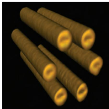
**Fig 1: A 3D reconstruction of a hexagonal waveguide array using third harmonic generation imaging techniques.**
