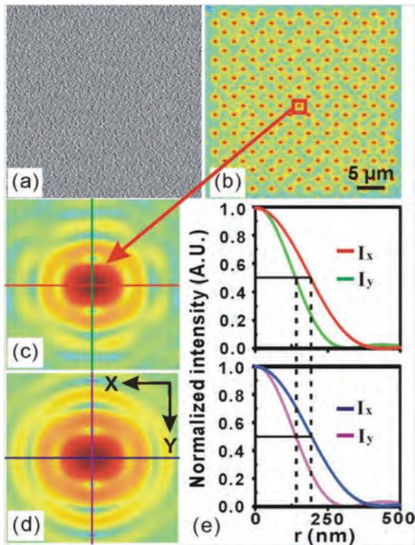
Fig 5: (a) Phase pattern consisting of  $1080 \times 1080$  (256 gray levels) pixels for a 200-spot array; (b) calculated intensity distribution from the phase pattern using the Debye integral; (c) density plot for one focal spot in the array; (d) density plot for a single focal spot; (e) intensity cross sections along the marked color lines of the spots. The scale bar is  $5 \mu\text{m}$ .
