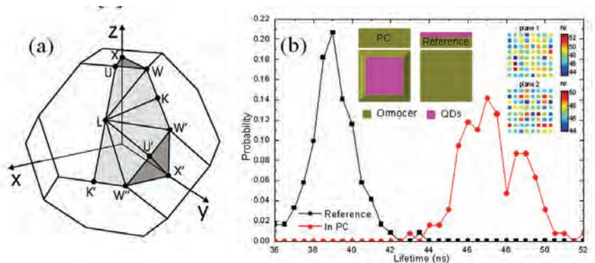
**Fig 1: (a) Brillouin zone for the woodpile PCs used in experiment. (b) Lifetime distributions measured in PCs and reference samples showing obvious inhibition of QD emission in PCs.**
