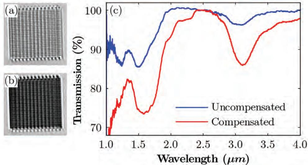
Fig 3: (a, b) Optical images of 32 layer, 4.5 μm lattice constant photonic crystals fabricated in lithium niobate, with and without compensation of the index mismatch aberration respectively. Fig. (c) Transmission spectrum of the two crystals, showing improvement in bandgap strength when compensation is applied.
