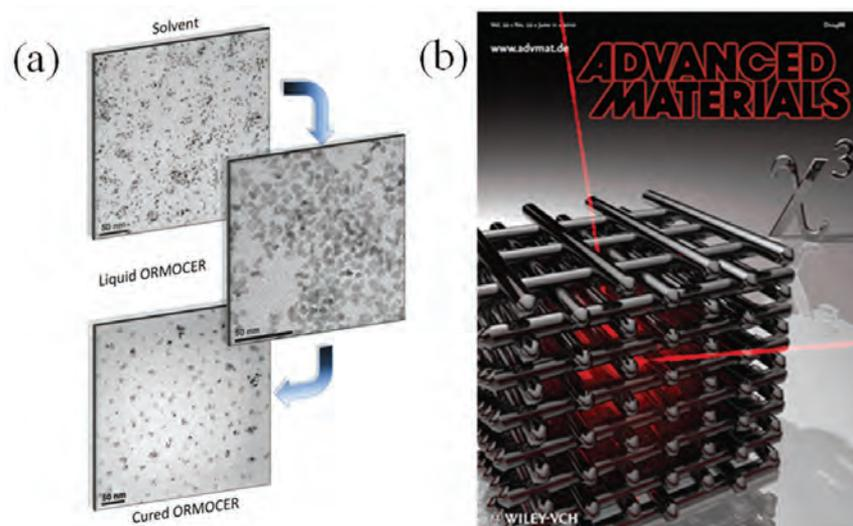
Fig 4: (a) A sequence of TEM images showing the QDs at each stage of the dispersion process. (b) The paper has been published on *Advanced Materials* and being selected as the cover story.
