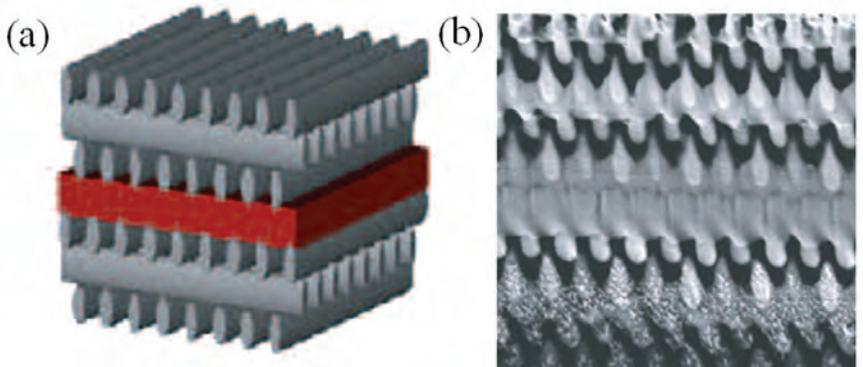
**Fig 2: (a) Sketch of 3D woodpile PC in ChGs with a planar defect in the middle. (b) SEM image of fabricated PC with the planar defect in the middle.**
