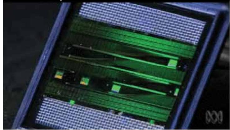
**Fig 4. Image of the 6 cm size  $\text{As}_2\text{S}_3$  optical chip fabricated at ANU, consisting of a series of straight and serpentine shaped planar waveguide of various rib widths for tailoring the total dispersion to enable broader bandwidth signal processing. Source: ABC Catalyst (03/09/2009) (<http://www.abc.net.au/catalyst/stories/2675781.htm>)**
