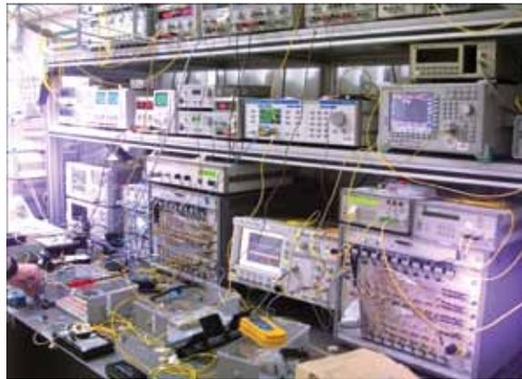
**Fig 3. High-speed optical communication facility for generating, transmitting and detecting high-speed data signals with serial bit-rate up to 640 Gb/s. This system enables the testing of the bit-error rate performance of the nonlinear optical devices in broadband signal processing applications.**
