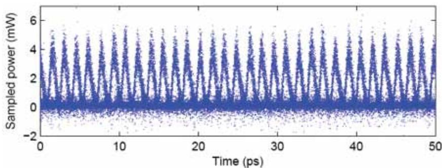
**Fig 6. Optical sampling using a dispersion-shifted  $As_2S_3$  waveguide for the nonlinear medium, to generate a high resolution “eye diagram” trace of a 640 Gb/s optical signal.**
