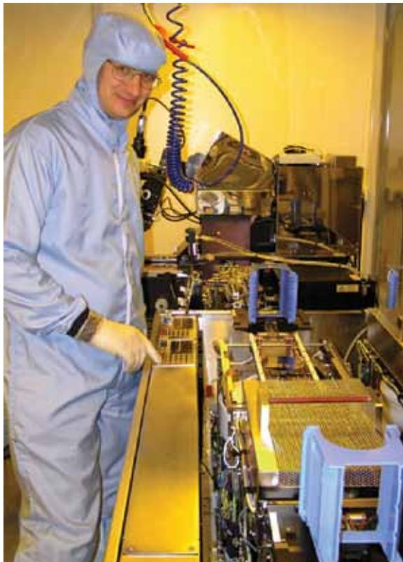
**Fig 2. Steve Madden using track coating and lithography tools for chalcogenide waveguide fabrication.**
