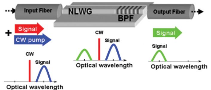
**Fig 1. Concept of a phase preserving wavelength converter based on CW pumped FWM by the ultra-fast optical Kerr effect in a nonlinear waveguide (NLWG), which has a bandpass optical filter (BPF) integrated in the same device.**
