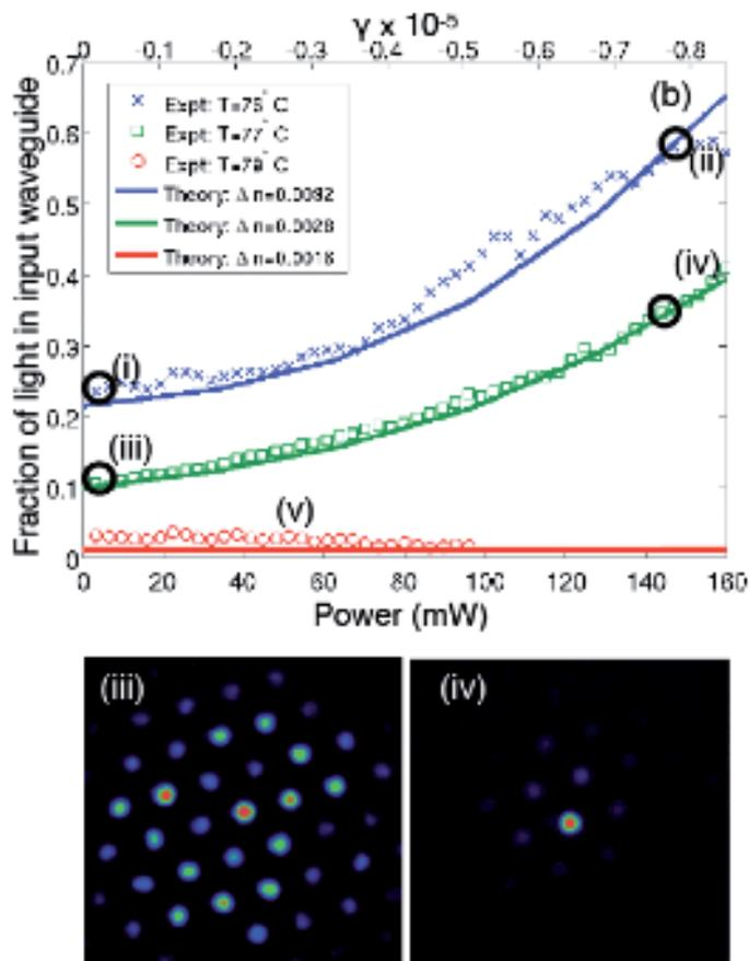
**Fig 1. (Top) Fraction of light into the input waveguide with increase of the incoupling power, for three different temperatures (refractive index contrast) of the system. (Bottom) typical intensity profiles for the point (iii) and (iv) as marked on the plot on the top.**
