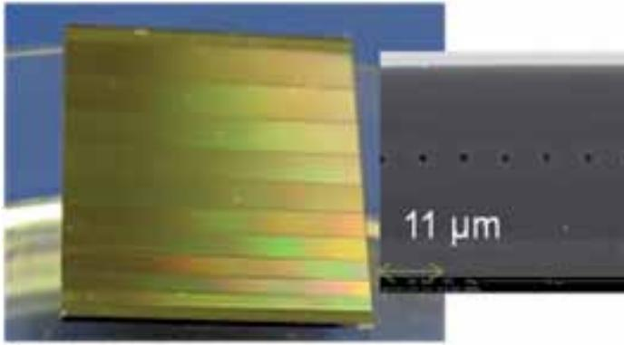
**Fig 2. Top view (left) and SEM image (right) of the polymer waveguide array before infiltration.**
