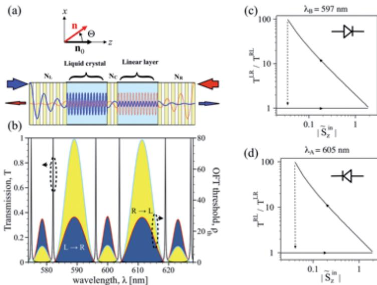
**Fig 3. Reversible optical diode based on double photonic crystal cavity infiltrated with liquid crystal. (Left) The variation of the Fréederickz threshold inside the photonic band gap for light impinged from different directions. (Right) The ratio of transmission coefficients in opposite directions at different wavelengths.**
