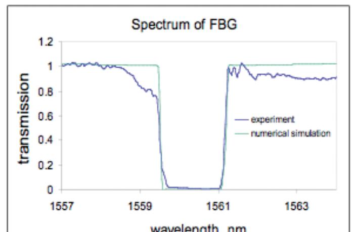
**Fig 2. Transmission spectrum of an apodized FBG written in a chalcogenide  $\text{As}_2\text{S}_3$  rib waveguide.**
