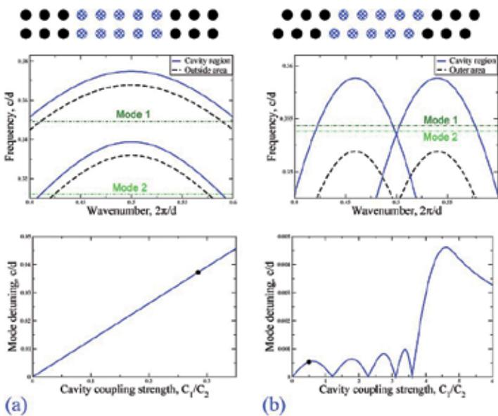
**Fig 4. Tuning of coupled-cavity modes in with (a) zero lateral displacement and (b) half-period shift. Middle row: wave dispersion inside and outside the cavity region, and the frequencies of fundamental cavity modes. Bottom row: dependence of the mode detuning on the transverse coupling strength.**
