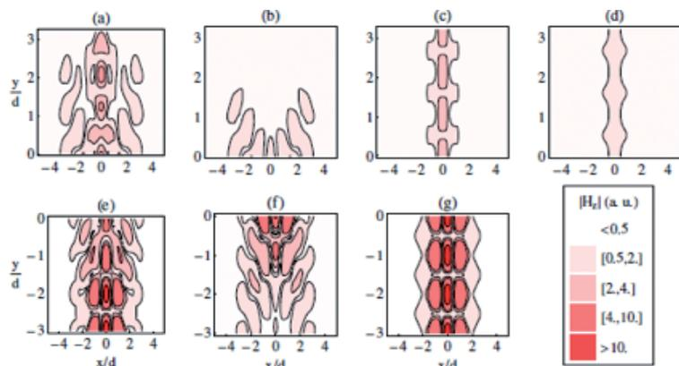
**Fig 1. Magnetic field versus position when light is incident from a fast waveguide onto a slow one. The top row (a-d) refers to the field in the fast medium while the bottom (e-g) refers to the slow medium. Shown are: the total field (first column a,e), the evanescent field (second column b,f), field of the forward propagating modes (third column c,g), field of the backward propagating mode (fourth column d).**
