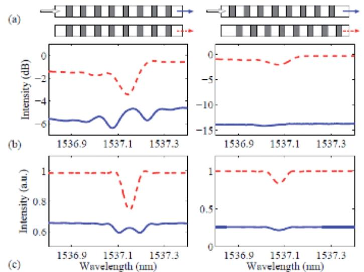
**Fig 5. (a) Schematics of symmetric (left column) and antisymmetric (right column) Bragg-grating couplers. (b) Measured and (c) calculated transmission spectra from first (solid) and second (dashed) waveguides when the light is coupled to the first waveguide.**
