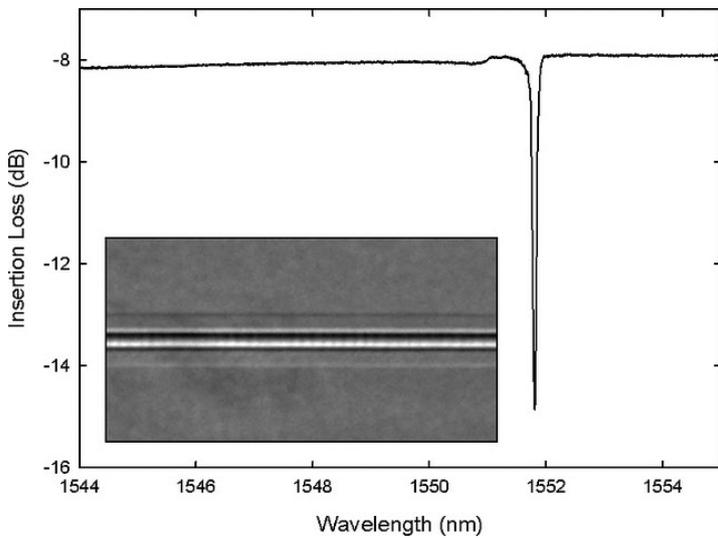
**Fig 4. Transmission spectrum from a 1st order waveguide Bragg grating fabricated in undoped borosilicate glass using a high power oscillator. Inset shows an optical micrograph of the waveguide Bragg grating structure.**
