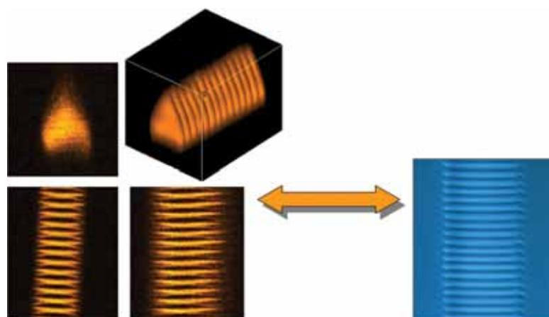
**Fig 2: (left) Third harmonic generation (THG) projections of a 2  $\mu\text{m}$  period waveguide Bragg grating written in Yb-doped phosphate glass and (right) a transmission differential interference contrast (TDIC) image of the same structure.**
