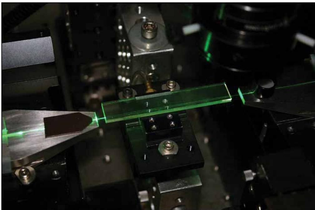
**Fig 1. Photo-annealing ultrafast laser written waveguide Bragg gratings in Yb-doped phosphate glass using 532 nm light.**
