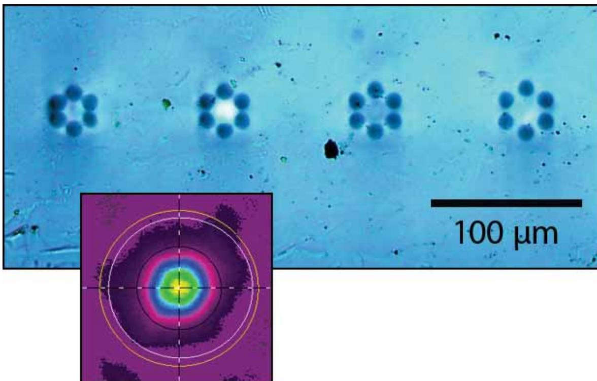
**Fig 5. Optical micrograph illustrating depressed cladding arrangements of negatively induced refractive index channels going into the page. Inset shows a circular 1550 nm mode that guides down the centre of one of the depressed cladding arrangements.**
