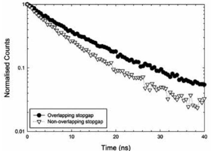
Fig 4. Time-resolved fluorescence measurements of the NV centers inside opals.
