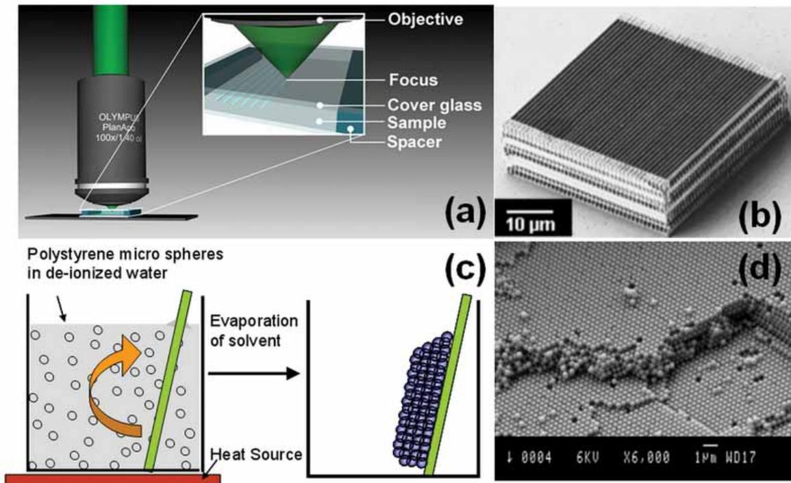
**Fig 1. Schematic drawing of (a) the DLW setup and (b) a woodpile 3D PC generated by DLW in high index chalcogenide glasses. (c) Self-assembly setup and (d) opal PC generated by self-assembly.**
