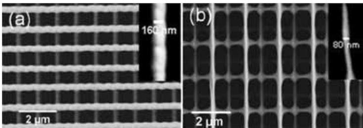
Fig 2. SEM images of chalcogenide PCs fabricated with high (left) and low (right) repetition rate laser beams.
