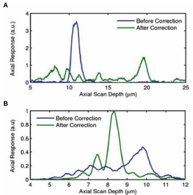
**Fig 6. Axial response showing adaptive optics compensation result at (a) low laser power and (b) high laser power.**
