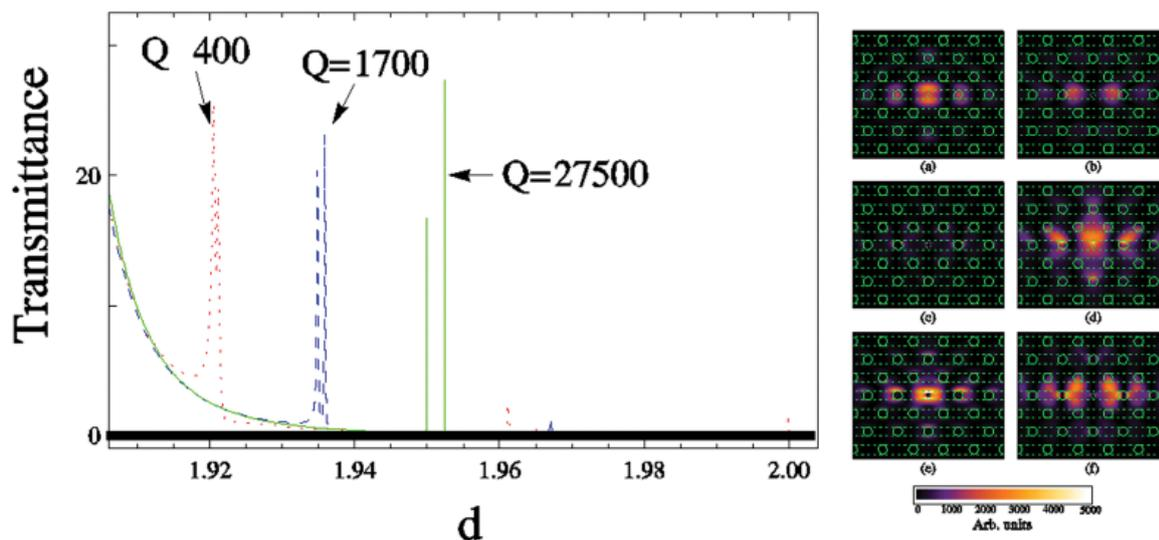
Fig 7. Q factor of the defect states and their field distribution
