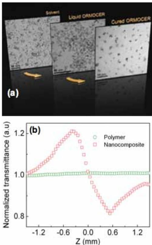
**Fig 5. (a) Transmission electron microscopic images showing the process and quality of the QDs and nano-composites. (b) closed-aperture Z-scan results at 800 nm for the nanocomposites.**
