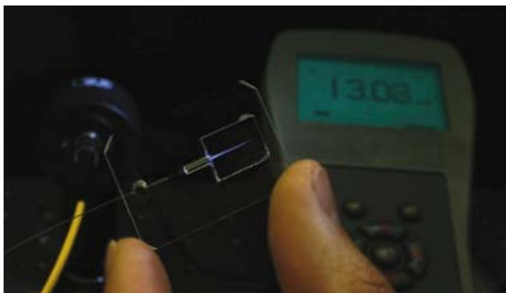
**Fig 2. Fibre pigtailed monolithic Yb doped DFB waveguide laser operating at 1  $\mu\text{m}$ , fabricated using direct write techniques. Note the power reading in the background. Inset: Difference interference contrast micrograph of a waveguide Bragg grating inscribed inside Er-Yb doped phosphate glass. The period is  $\sim 500$  nm, suitable for feedback at 1.5  $\mu\text{m}$ .**
