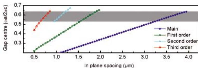
**Fig 1. The mid-gap position for different order band gap as a function of the in-plane spacing.**
