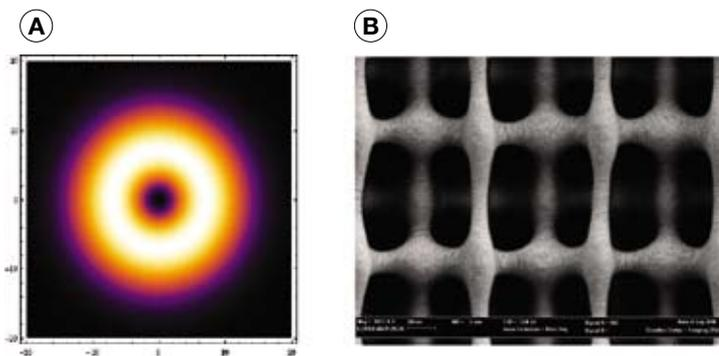
**Fig 2. (a). Radially polarised beam (b). SEM image of 3D woodpile structure fabricated using the radially polarised beam.**
