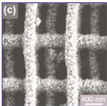
**Fig 5. The cartoon of 3D woodpile photonic crystals before (a) and after (b) the infiltration. (c) The SEM image of silver nanoparticle coated woodpile PhCs.**
