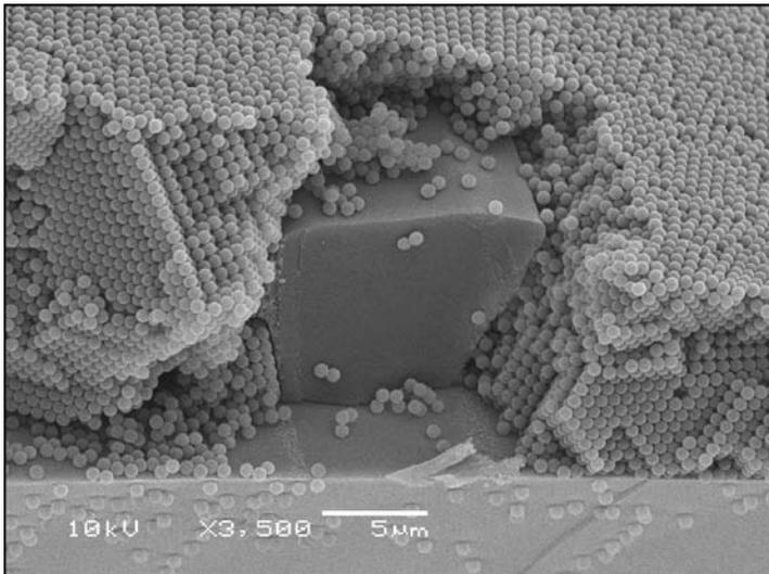
**Fig 2. Scanning electron micrograph of Su-8 waveguide on silicon substrate, with silica opal on the sides and top, showing good regularity of the photonic crystal structure.**
