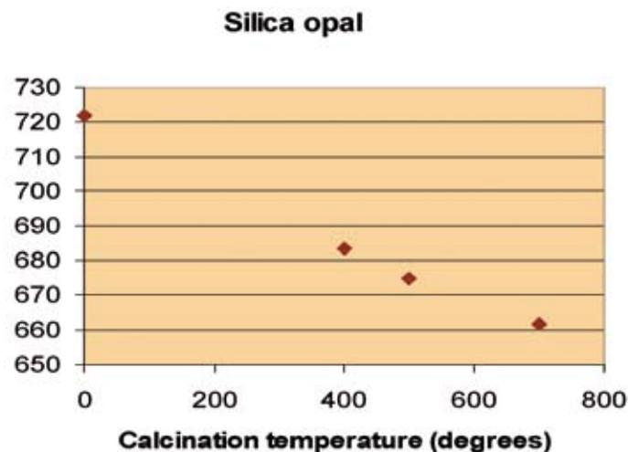
Fig 1. Stopgap peak wavelength as a function of annealing temperature for silica opal. The samples were heated for 3 hours.
