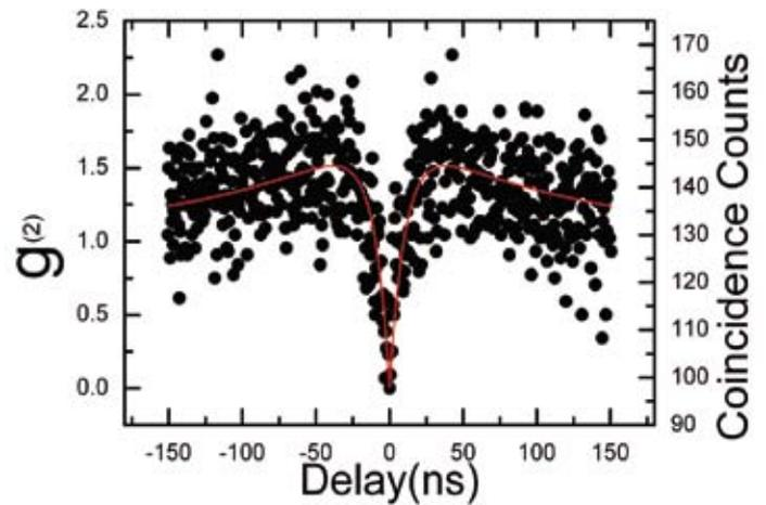
**Fig 5. Photon coincidence measurement and normalised second order correlation function of a single N-V centre in nanodiamond in polystyrene opal. The measurements indicate that the emitter is a single photon source.**
