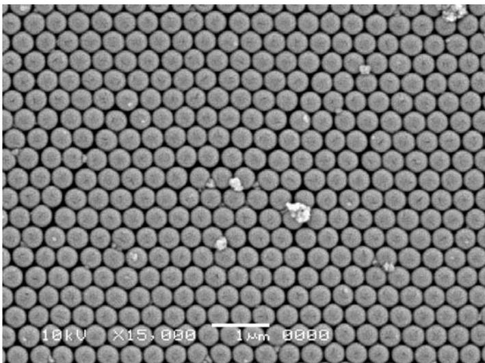
**Fig 3. Scanning electron micrograph of nanodiamond particles on the surface of a polystyrene opal.**
