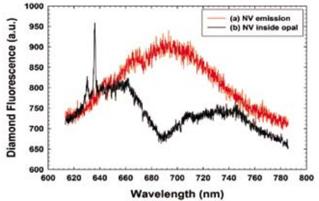
**Fig 4. Emission spectra for N-V centres in nanodiamonds on a silica substrate (red) and embedded in opal with a partial bandgap at 690 nm (black).**
