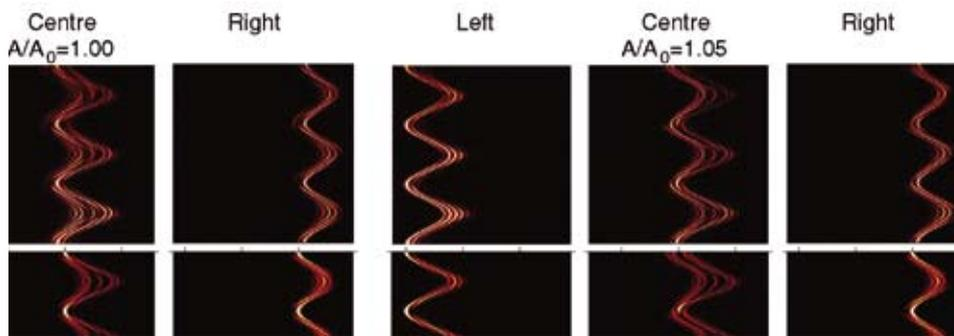
**Fig 1. (a,b) Light propagation in the two curved arrays with different bending amplitude  $A$ . In each of the two blocks experimental fluorescent images are shown on the top, and corresponding numerical simulations are shown at the bottom. Light is launched into the left edge waveguide of the array (left), center waveguide (center), and right edge waveguide (right).**
