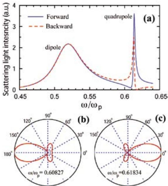
**Fig 4. Exact Mie solution of the light scattering by a plasmonic nanoparticle. The radius of the nanoparticles is much smaller than the light wavelength. (a) Frequency dependence of the scattering light intensity in the vicinity of the dipole and quadrupole resonances. In the latter case both forward (solid lines) and backward (dashed lines) scattering profiles exhibit asymmetric Fano resonances; (b,c)**
