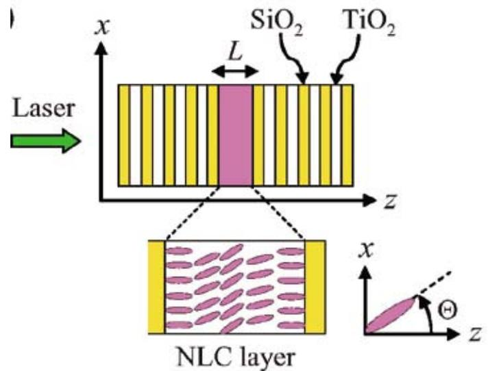
**Fig 5. Sketch of the multilayers periodic structure with an embedded nonlinear liquid crystal defect.**
