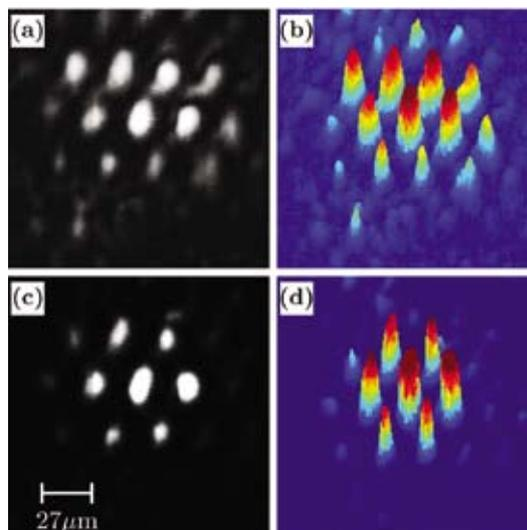
**Fig 2. Output intensity distributions and corresponding three-dimensional surface plots of the probe beam for (a,b) low input intensities and (c,d) high input intensities.**
