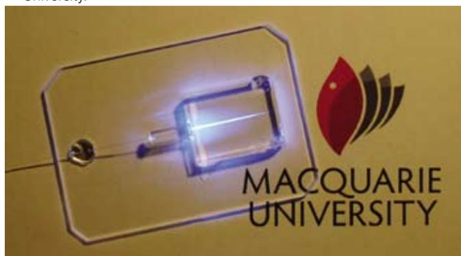
**Fig 1.** Image shows the monolithic Yb doped DFB waveguide laser. The device is single-end pumped from the left via a pigtailed diode laser. Due to the presence of an asymmetric phase change the bulk of the output power is directed to back into the fibre pigtail. Note the characteristic blue cooperative luminescence in the Yb doped host glass.
