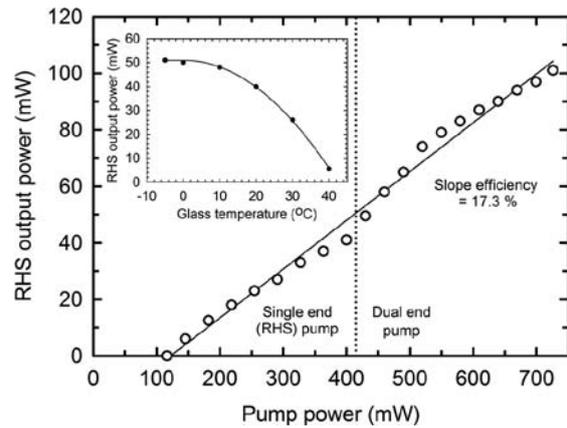
**Fig 2. Output power of a 9.5 mm, 1032 nm waveguide laser at room temperature, as a function of pump power for single- and dual-end pump geometries. Inset shows the effect of bulk glass temperature on laser output power.**
