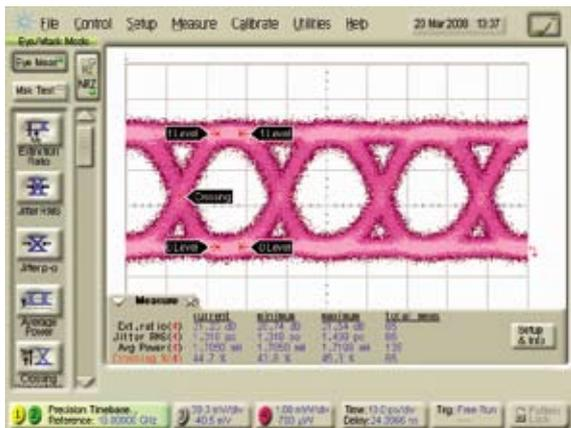
**Fig 3. Eye-diagram from the first measurements of error-rates in a packaged laser written amplifier performed in collaboration with the University of Sydney node. The amplifier device showed no significant system penalty.**
