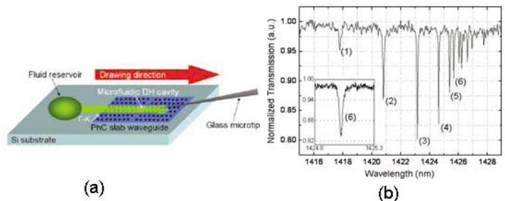
**Fig 1. (a) Infiltration schematic: a glass micro-tip is used to draw the infiltration fluid across the PhC section, forming the DH stripe. (b) Transmission spectrum of a microfluidic double heterostructure cavity in Si. Inset, close-up view of resonance (6). The intrinsic Q is around 60000.**
