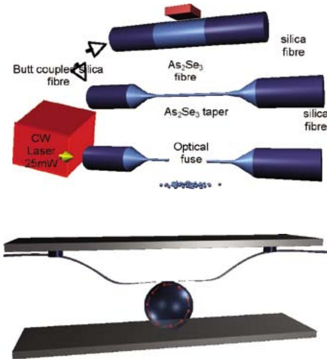
**Fig 4. (a) Fabrication process, (b) coupling setup between a silica taper and a microsphere**
