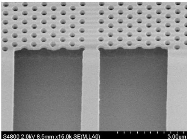
**Fig 5. SEM picture of a photonic crystal waveguide connected to a nanowire in AMTIR1 recently produced at St Andrews**
