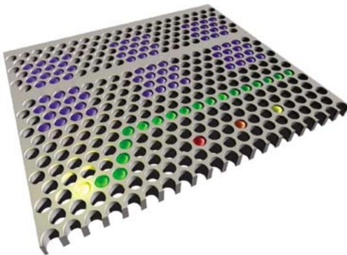
**Fig 2. Schematic vision of the “reconfigurable optofluidics photonic chip”**
