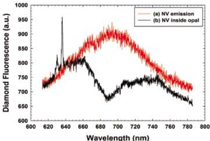
Fig 5. Emission spectra of N-V centres in nanodiamonds on a silica substrate and incorporated into a silica opal with stopgap ~690 nm.
