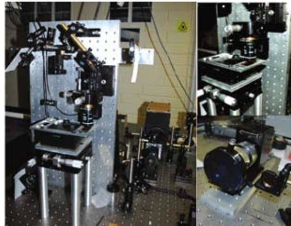
**Fig 9. The experimental setup for aberration compensation in DLW in high-index materials.**
