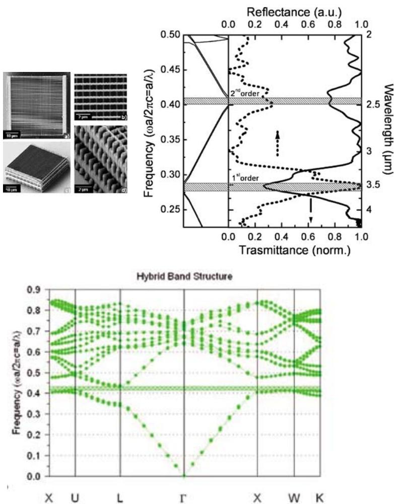
Fig 7. (a): SEM image of 3D chalcogenide PCs with different lattice constant. (b) Left: Calculated band structure of a 3D woodpile PC predicting the presence of both the first and the second order stop gaps. (b) right: Measured transmission and reflection spectra of the 3D woodpile PC matching exactly the calculation. (c) Calculated band structure of a 3D PC showing a complete bandgap.
