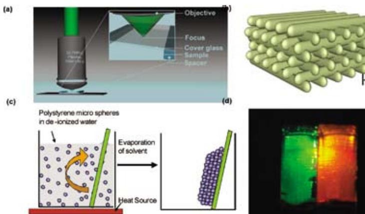
**Fig 2. Schematic drawing of (a) the DLW setup and (b) a woodpile 3D PC generated by DLW. (c) Self-assembly setup and (d) two opal PCs generated by self-assembly.**
