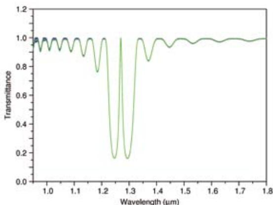
Fig 6. Transmittance spectrum for a woodpile consisting of 40 layers of polymer rods on either side of an air-gap defect. The size of the air-gap has been optimised so that the frequency of the defect mode occurs at the centre of the bandgap for the woodpile.
