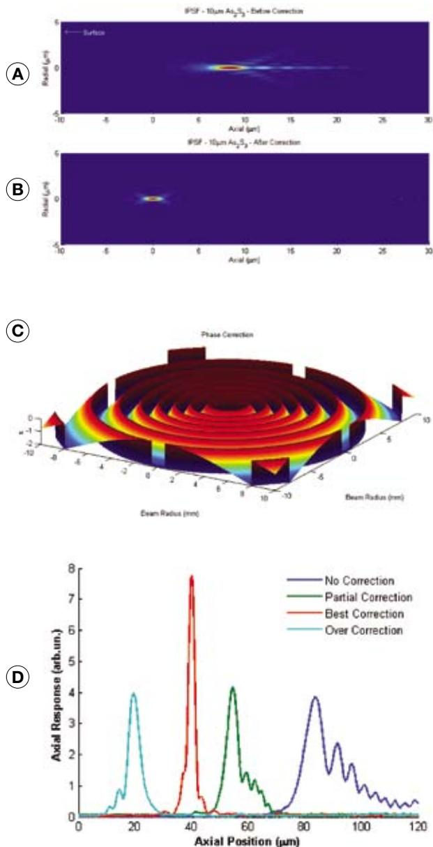
**Fig 8. (a) The degraded focal spot caused by strong aberration. (b) The nice and clean focal spot after aberration compensation. (c) A typical pre-designed phase pattern to compensate the aberration in chalcogenide glasses. (d) Axial response showing the effect of aberration compensation.**
