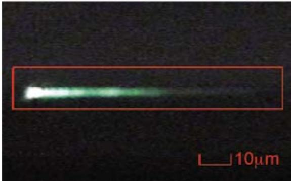
**Fig 2. (a) Scanning Electron Micrograph of a dispersion engineered slow light photonic crystal waveguide connected to a nanowire. (b) Green light obtained through third harmonic generation occurring in the photonic crystal waveguide (highlighted as the red box) and measured on a CCD camera.**
