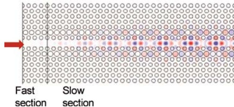
**Fig 4. Field distribution corresponding to the transmission from a regular "fast" waveguide (left of the interface) into a slow-light waveguide (right hand side). An efficient coupling is visible without any transition region.**
