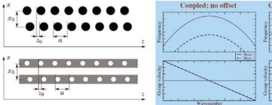
**Fig 5: Results of the analytical prediction of the universal dependence of slow-light dispersion (right) for coupled periodic waveguides with different longitudinal offsets. The model is valid for both geometries displayed on the left [4].**
