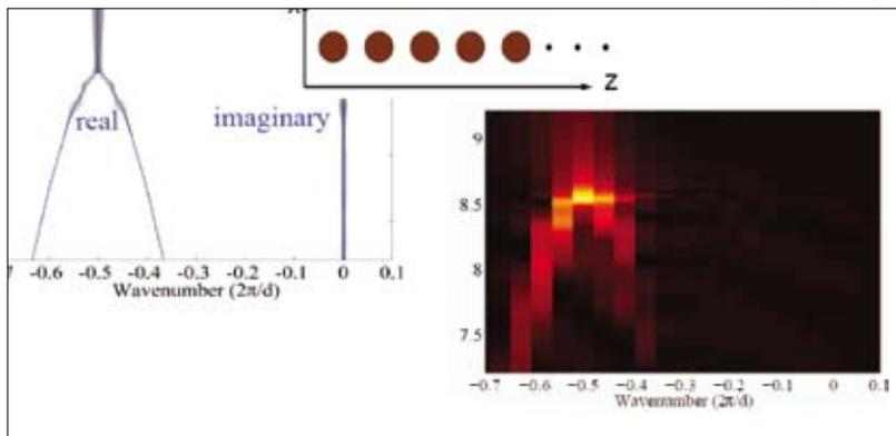
**Fig 6: Left: dispersion in a periodic waveguide, extracted from experimental near-field measurements using an original approach. The spectral resolution is dramatically improved compared to the spatial Fourier transform method presented on the right.**
