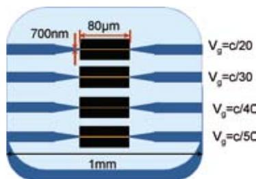
**Fig 3. (a) Schematic of the silicon chip including a series of dispersion engineered photonic crystal waveguides with different group velocities. (b) Associated transmission through these waveguides which shows a saturation effect at high power that is related to nonlinear absorption and is enhanced at lowest group velocities [2].**
