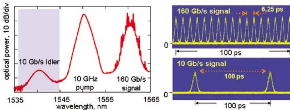
**Fig 7. Demonstration of low power (25 mW) time-division demultiplexing of a 160 Gb/s signal in a 5 cm length tapered  $\text{As}_2\text{S}_3$  fibre (a) Output optical spectra showing generation of a 10 Gb/s idler by FWM between the signal and 10 GHz pump pulse train, and (right) high-speed sampling scope images of (b) (upper) 160 Gb/s input signal and (lower) 10 Gb/s tributary channel contained in the FWM idler after optically filtering the waveguide output spectrum.**
