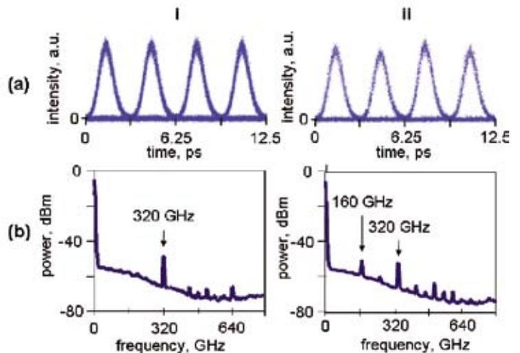
**Fig 6. Broadband measurement traces of 320 Gb/s signals generated by either (i) optimum or (ii) non-optimum time-division multiplexing when captured as (a) “eye diagrams” from a high resolution optical sampling scope and (b) RF spectra from the photonic chip based RF spectrum analyser, which reveals amplitude modulation distortion at 160 GHz frequency.**
