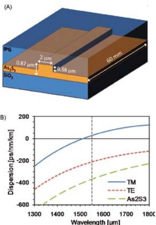
**Fig 4. (Top) device illustration of a 6 cm length dispersion-shifted  $\text{As}_2\text{S}_3$  planar waveguide of  $2 \mu\text{m}$  rib width and (bottom) calculated group velocity dispersion of fundamental TM and TE modes compared to material dispersion of  $\text{As}_2\text{S}_3$ , highlighting the dispersion-shifted design enabled by reducing the  $\text{As}_2\text{S}_3$  film thickness**
