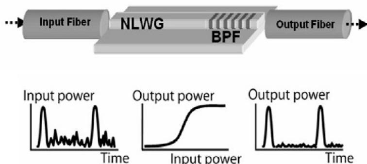
**Fig 1. All-optical signal regenerator concept exploiting optical Kerr effect in nonlinear waveguide (NLWG), which has a bandpass optical filter (BPF) integrated in the same device.**
