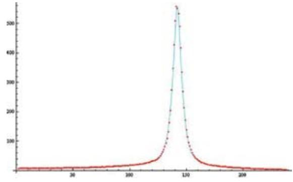
**Fig 5: A plot of flux vs radius in pixels for a fibre with a surface roughness of 45nm rms. Red points are the data, blue line is a Voigt fit to the data. The Voigt fit is a significant improvement over the Gaussian fit.**
