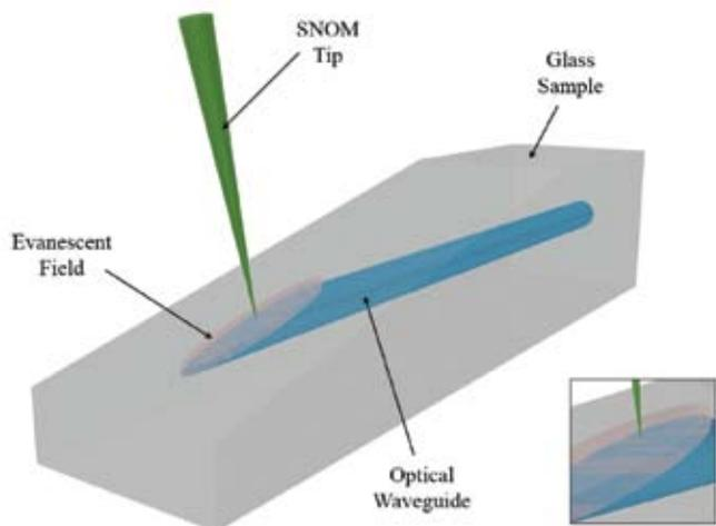
**Fig 3: Schematic illustrating probing of ultrafast laser written embedded waveguides using Near-field Scanning Optical Microscopy.**
