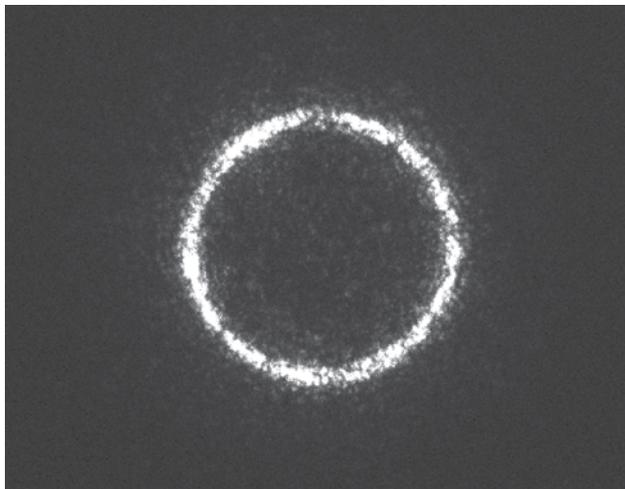
**Fig 4: Image of the far field light distribution of a fibre with 8nm rms surface roughness using a HeNe laser as the input light source.**
