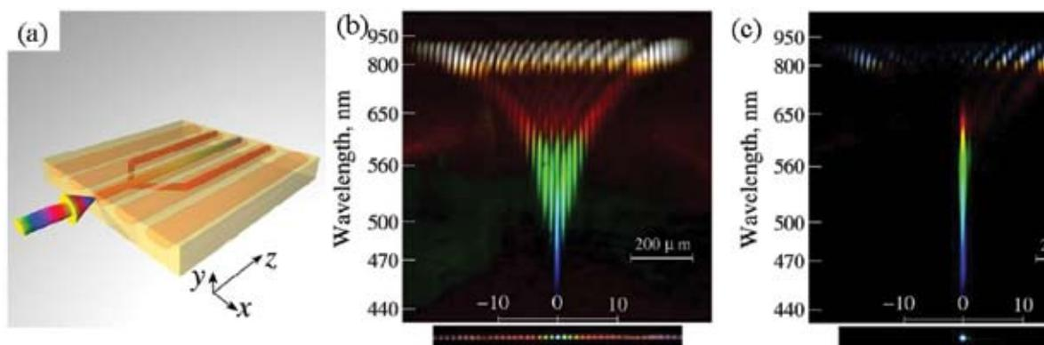
**Fig 2: Nonlinear spectral-spatial control and localization of supercontinuum radiation. (a) Schematic of the experiment illustrating the dispersion of the colors inside the array of optical waveguides. (b) Spectrally resolved diffraction of the supercontinuum radiation (low input power of 17  $\mu$ W). (c) Spectrally resolved localization of the supercontinuum inside the central waveguide at input power of 7.5 mW Bottom in (b-c): output color intensity profile.**
