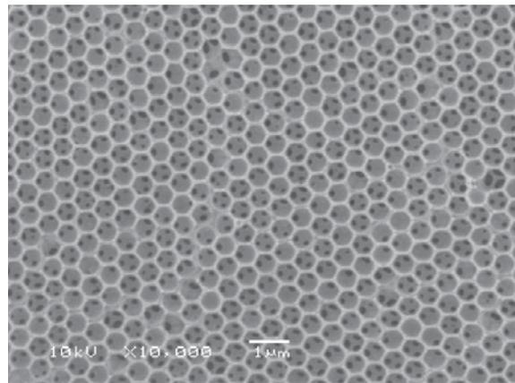
**Fig 4: An inverse opal structure showing periodicity over large areas.**
