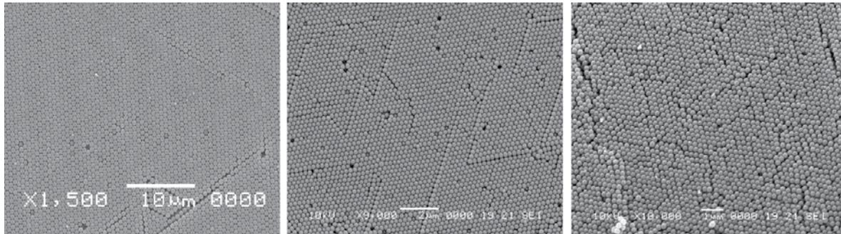
**Fig 2: SEM images of opals grown on various surfaces: (a) flat surface, (b) capillary and (c) optical fibre. It is obvious that as the substrate curvature increases, the periodicity of the top layer of spheres gets worse.**
