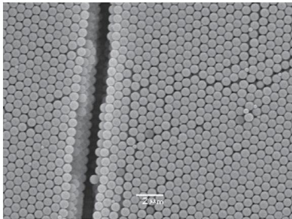
**Fig 3: A 3D photonic crystal made of polymer microspheres arranged in a face centred cubic symmetry.**
