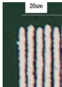
**Fig 5: Gold film on glass substrate with laser-micro-machined lines etched to create nano-wires for plasmonic waveguides.**
