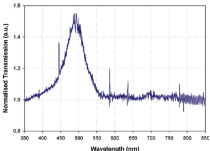
**Fig 1: Wavelength specific increase in opal clad fibre transmission. The position of the increase corresponds to the position of the photonic bandgap.**
