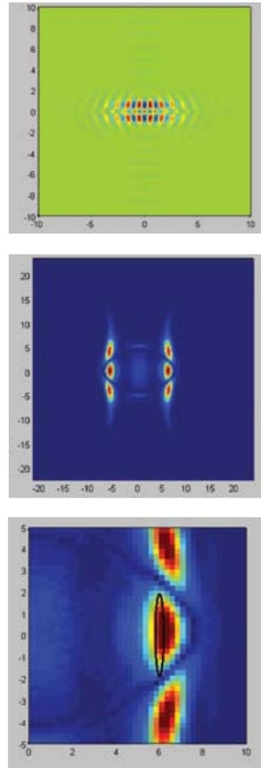
**Fig 4a):** Calculated defect state. **b):** Representation of the defect in reciprocal space. **c):** Close up of the reciprocal space overlap between the defect state and (black contour) the fundamental mode of a silica fibre taper.
