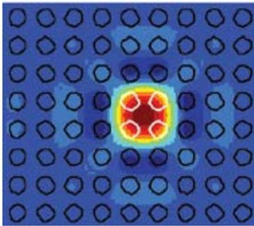
**Fig 5: The four defect modes of a square defect (comprising the four cylinders in white whose dielectric constant has been varied) in a square lattice. The mode symmetries follow in a straightforward manner from the solution of the eigenproblem for a circulant matrix.**
