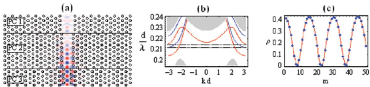
**Fig 1: (a) Schematic of the coupling structure; (b) Band structure for PC 1 (red) and PC 3 (blue); (c) Reflectance  $\rho$  of the entire optimized structure versus  $\mu$ , the length of PC 2.**
