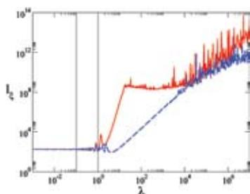
**Fig 6: Localization length as a function of wavelength for normal materials (blue) and for mixed stacks (red), clearly showing the  $\lambda^2$  and  $\lambda^6$  dependence for refractive index disorder.**
