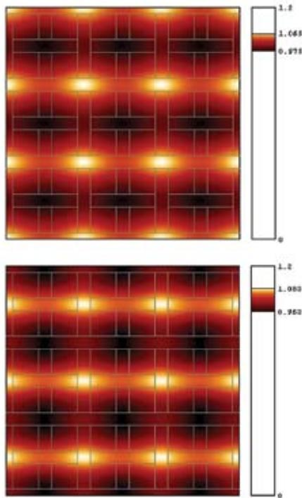
**Fig 3:** Near field intensity plots at the exit face of a woodpile PC at frequencies just below (left) and just above (right) the bandgap, showing the respective concentration of the fields within the rods and within the voids between them.
