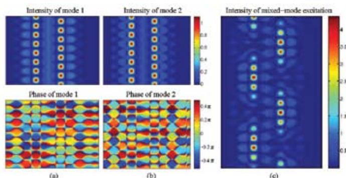
**Fig 1: Slow-light waveguide coupler. (a,b) Intensity (top) and phase (bottom) of the transverse magnetic field distributions for the band-edge modes of antisymmetric coupler with (a) positive and (b) negative wavenumbers, respectively. (c) Intensity of the simultaneously excited modes.**
