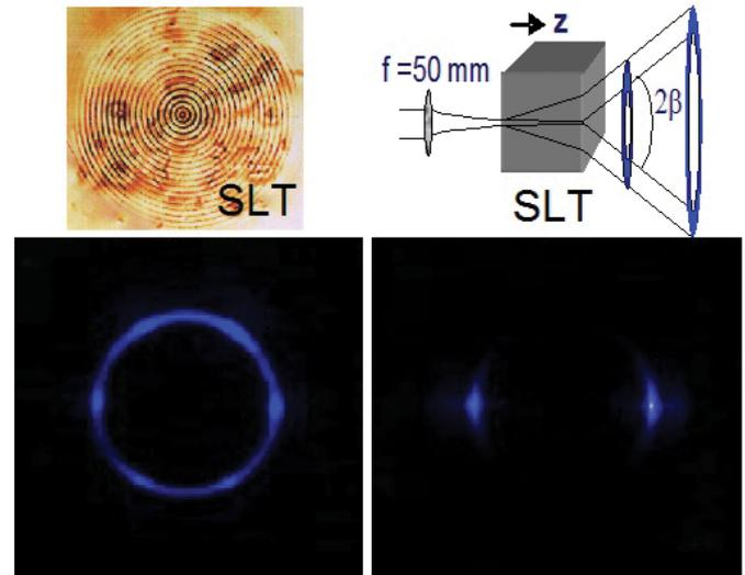
**Fig 3: Second-harmonic generation by annularly poled structures. Above: Front facet of the annular periodically poled Stoichiometric Lithium Tantalate (SLT) sample and schematic of the experiment. Below: far-field image of the second-harmonic rings.**
