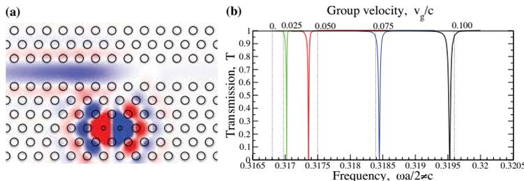
**Fig 2: All-optical switching of slow light. Double-defect waveguide-cavity structure with the cavity created by two defect rods. (a) Electric field at the resonance reflection, (b) Transmission spectra for different values of the radius**
