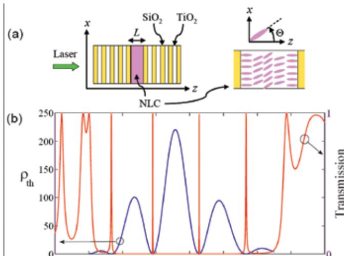
**Fig 2: Spectral modulation of the Freedericksz transition: a) a periodic structure, consisting of alternating layers of  $\text{SiO}_2$  and  $\text{TiO}_2$ , contains a liquid crystal defect. Molecules of liquid crystal orient along the rubbing direction; b) it is possible to observe first (blue) or second (red) order types of transition for the same liquid crystal, depending on the pumping wavelength.**
