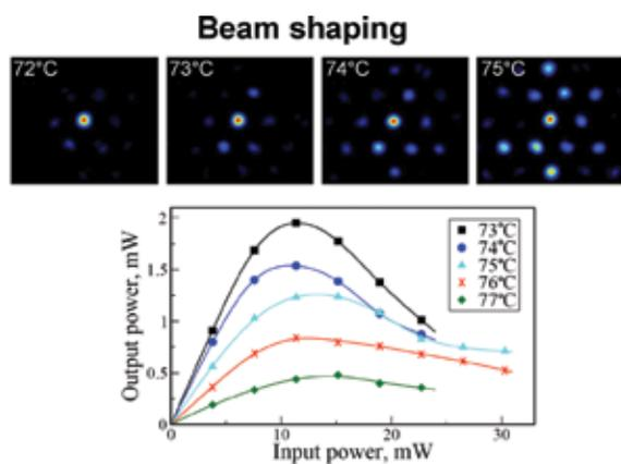
**Fig 1: Photonic crystal fiber with solid core, surrounding holed fluid infiltrated Images: linear output intensity distribution at various temperatures; graph: non-linear behavior with output power in the central waveguide varying as a function of input power at each different temperature [1].**
