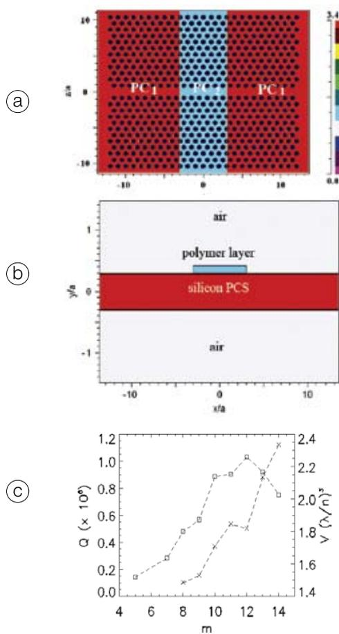
**Fig 3: (a) Top view of a double heterostructure cavity; PC2 has slightly higher average refractive index than PC1. The black holes are air holes. (b) Silicon slab with polymer strip on the top; (c) total Q (rectangles) and modal volume V (crosses) versus the cavity width m, the inset shows the PCS cross-section.**
