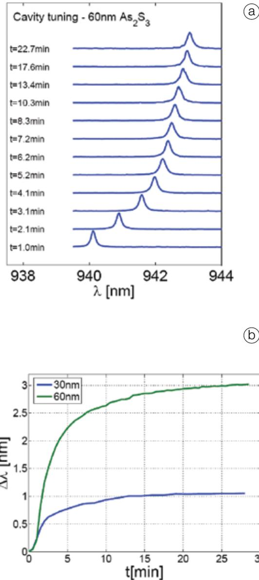
**Fig 4: (a) Spectra showing the shift of the cavity resonance because of the photodarkening of the 60nm thick chalcogenide layer. (b) Time dependence of the cavity resonance for 60nm and 30nm  $As_2S_3$ .**
