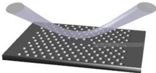
**Fig 1: Coupling scheme used: schematic showing the coupling from a tapered fibre to PhC nanocavity**
