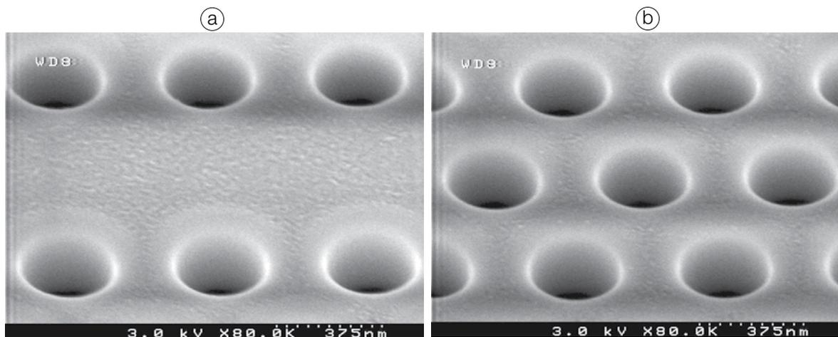
**Fig 5: SEM micrograph of a) a photonic crystal L3 cavity b) a photonic crystal waveguide fabricated by FIB milling**
