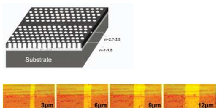
**Fig 2: Top: Schematic of a DH cavity created from the infiltration of liquid into a defined area of a photonic crystal lattice. Bottom: A W1 PCS structure exhibiting increasingly wider microfluidic DH cavities.**
