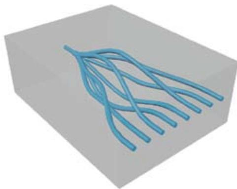
**Fig 2: The rendered drawing of a 1-to-8 three-dimensional waveguide splitter. The design pictured above was directly used to fabricate the splitter and is not an artistic impression.**
