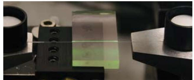
**A waveguide laser device being tested at CUDOS Macquarie University. The active waveguide region glows green under optical pumping.**
