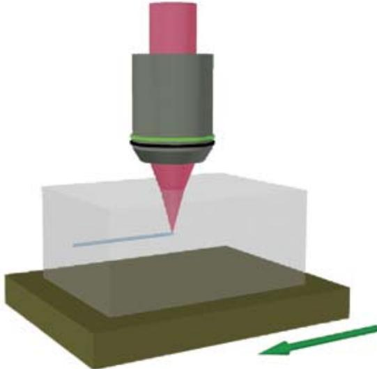
**Representation of the direct write method. A femtosecond laser beam is focused inside a moving dielectric material sample to create a permanent optical waveguide.**
