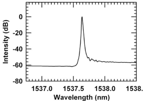
**Fig 1: Output spectrum from a WGL. The width of the laser line is limited by the 10 pm OSA slit width.**
