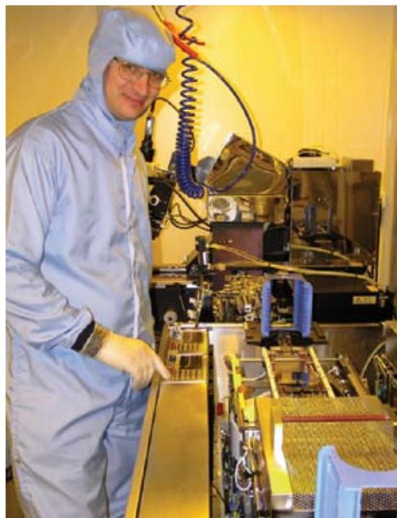
**Fig 2: Steve Madden using track coating and lithography tools for chalcogenide waveguide fabrication.**
