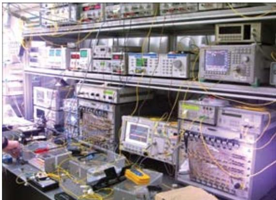
**Fig 3: 160 Gb/s facility and eye diagram of 160 Gb/s optical signal measured on high-speed sampling-oscilloscope for testing bit-error rate performance of nonlinear optical devices.**
