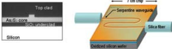
**Fig 4: (Left) Scanning Electron Microscope image of the low loss Chalcogenide planar waveguide fabricated from a thermally deposited film of  $As_2S_3$  and (right) device illustration showing the 22.5 cm long serpentine shaped rib of 4  $\mu m$  width.**
