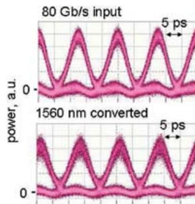
**Fig 6: High-speed sampling oscilloscope showing eye diagrams of an 80 Gb/s signal undergoing wavelength conversion from 1550 to 1560 nm wavelength by optically filtering the XPM broadened spectra from a 22.5 cm long  $As_2S_3$  rib waveguide.**
