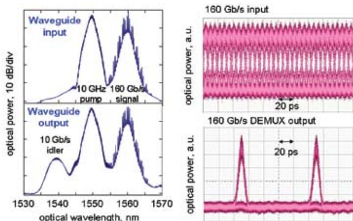
**Fig 7: (Left) Optical spectra at input and output of a 5 cm length  $\text{As}_2\text{S}_3$  rib waveguide showing generation of a 10 Gb/s idler by FWM between a 160 Gb/s signal and 10 GHz pump pulse train, and (right) high-speed sampling scope images showing 160 Gb/s time-division demultiplexing (DEMUX) operation by optically filtering the 10 Gb/s idler from the waveguide output spectra.**
