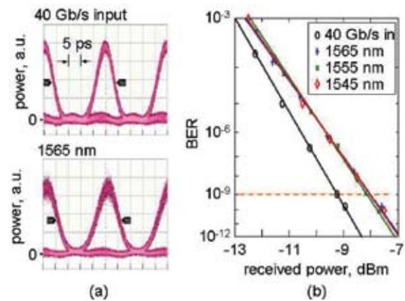
**Fig 5b: High-speed sampling oscilloscope showing eye diagrams of a 40 Gb/s signal undergoing wavelength conversion from 1535 to 1565 nm wavelength by optically filtering the XPM broadened spectra from a 22.5 cm long  $As_2S_3$  rib waveguide, along with the plot of its bit-error rate (BER) performance showing less than 1 dB power penalty at a BER of  $10^{-9}$ .**
