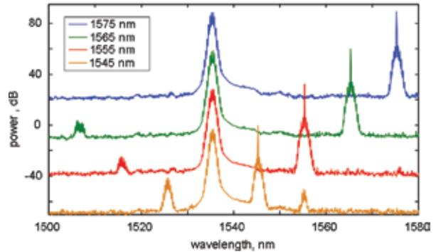
**Fig 5a: Output optical spectra from a 22.5 cm length  $As_2S_3$  rib waveguide showing the XPM of a 40 Gb/s signal (at 1535 nm wavelength) onto a co-propagating cw laser tuned to various wavelengths.**
