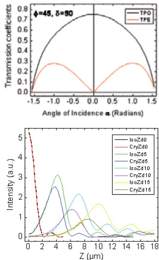
▲ Figure 3. (a) Transmission coefficients of o-rays and e-rays on the interface. (b) Comparison of the axial cross-section of the point spread function before and after taking into account of the anisotropy of lithium niobate.
