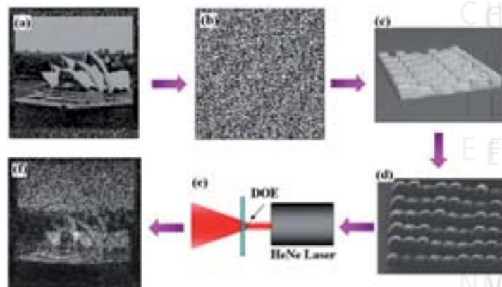
▲ **Figure 1.** (a) A 2D intensity distribution of a photo of the Sydney Opera House sampled by 128 x 128 points. (b) A designed phase profile for (a) with 256 phase levels by using the iterative Fourier transform algorithm. (c) A sketch showing an overall view of the designed DOE. The pixels are fabricated on a microscope cover glass. (d) A SEM image of the fabricated DOE. (e) Experimental setup for reconstructing the diffraction
