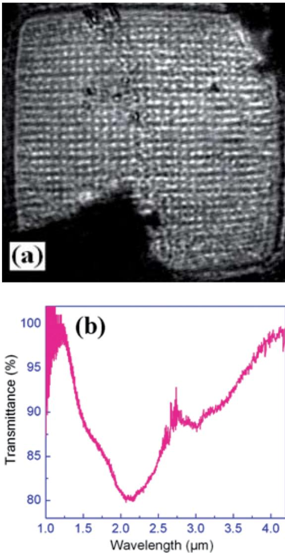
▲ Figure 2. Transmission confocal image of an inverse TiO<sub>2</sub> woodpile photonic crystal (a) and its transmission spectra (b).
