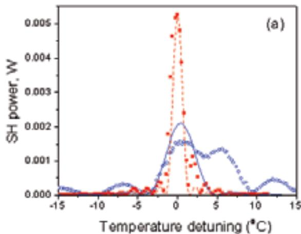
▲ Figure 2. Experimental (dots) and theoretical (lines) temperature phase-matching curves for SHG Type I (red) and SHG Type 0 (blue) in a 45.75 μm period gratings.
