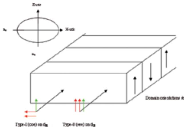
▲ **Figure 1. Schematic illustrating simultaneous, co-linear Type 1 and Type 0 nonlinear processes in periodically poled lithium niobate.**
