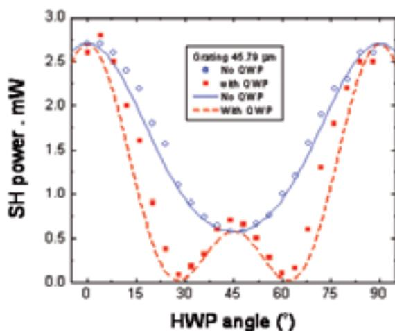
▲ Figure 3. Theoretical (lines) and experimental (dots) relationship between the SH power and the half-wave plate (HWP) angle which is controlling the input polarization. Blue traces indicate linear polarizations where only the HWP is in use. Red traces indicate elliptical/circular polarizations where a quarter wave plate is used in tandem with the HWP.
