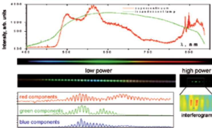
▲ Figure 2. Generation of a supercontinuum optical gap soliton. Top: spectrum of the generated supercontinuum, compared to the spectrum of white light lamp. Bottom: output intensity distribution for low laser power (left) and high power (right). Bottom right: interferogram demonstrating the staggered localized structure.
