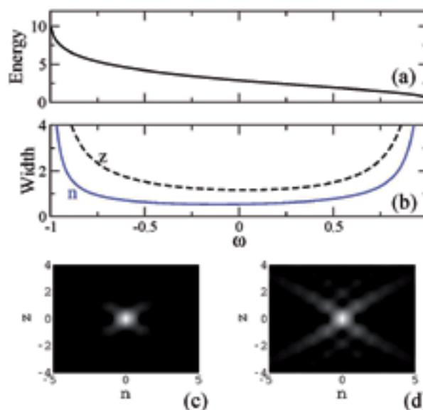
▲ Figure 1. Family of the light bullets characterized by (a) energy and (b) width along the transverse (solid) and longitudinal (dashed) directions vs. the frequency tuning inside the spectral gap. (c-d) Intensity profiles of two examples of slow-light optical bullets.
