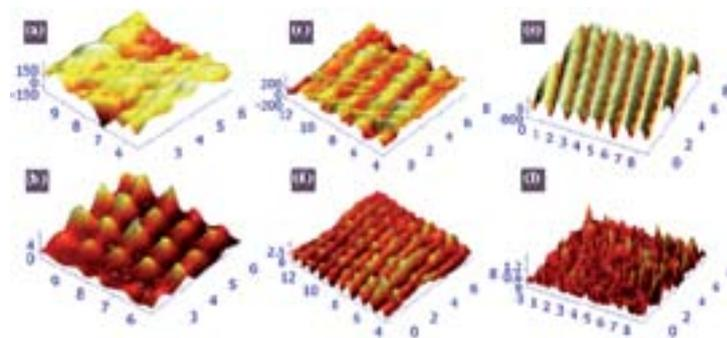
▲ **Figure 6. Topography signals (a, c, e) and optical signals (b, d, f) recorded simultaneously with a SNOM from 3D woodpile structures fabricated with different conditions. (a, b): The voids between the rods were totally filled with resin. (c, d): The voids between the rods were partially filled with resin. (e, f): A well-developed woodpile PC with a high quality PBG.**
