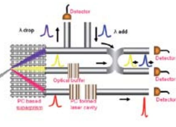
**▲ Figure 1. A schematic diagram for an all-optical chip consisting of photonic devices that may be fabricated by direct laser writing methods.**
