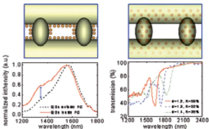
▲ Figure 4. Left column: Normalised photoluminescence spectra from quantum dots inside PC and outside PC at the same excitation condition. The arrow indicates the spectral redistribution in the shorter wavelength range. Right column: Transmission spectra of 3D PCs with different lattice constants  $d$ .  $R$  is the suppression ratio.
