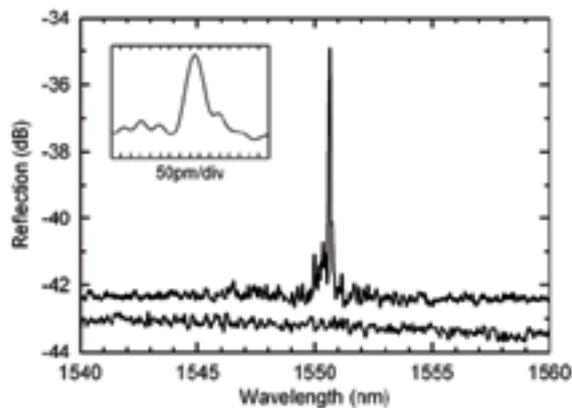
▲ **Figure 5. Reflection spectra from a waveguide Bragg grating (upper curve) and a waveguide-only structure (lower curve). The inset shows the WBG curve on an expanded abscissa.**
