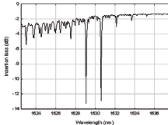
▲ **Figure 3. Sampled grating (50% duty cycle) with a  $\pi/2$  phase shift that suppresses the carrier wave.**
