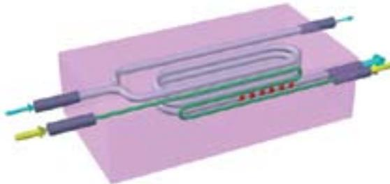
▲ **Figure 1. Conceptual illustration of an embedded waveguide amplifier written in rare earth doped bulk glass. This device includes evanescently coupled signal and pump waveguides, and an intra-core grating.**
