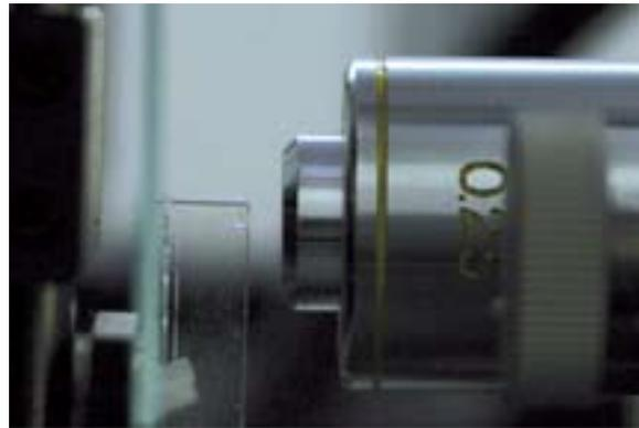
▲ **Figure 2. Enlarged image of a waveguide being written sub-surface in a glass sample by femtosecond laser light.**
