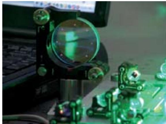
▲ **Figure 6. One of the key-elements of the chirped-pulse oscillator, a 2-inch diameter dielectric mirror which forms part of a so-called Herriott-cell, used to increase the resonator length to more than 27 m. Eight intracavity laser spots can be seen around its circumference.**
