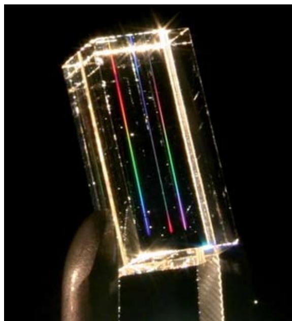
▲ **Figure 4. Image showing a set of waveguide Bragg gratings fabricated inside a block of fused silica. The visible light is produced by diffraction off the intra-core point-by-point grating.**
