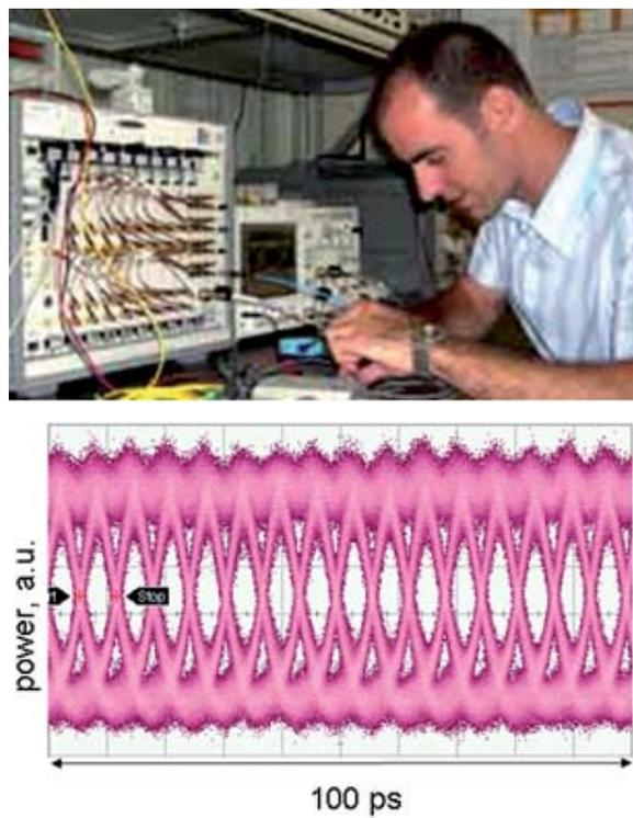
▲ **Figure 3. 160 Gb/s facility and eye diagram of 160 Gb/s optical signal measured on high-speed sampling-oscilloscope for testing bit-error rate performance of nonlinear optical devices.**
