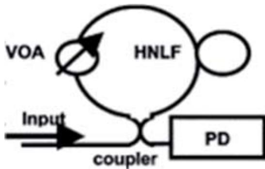
▲ Figure 4a. An OSNR monitor schematic using a highly nonlinear fibre (HNLF) and variable optical attenuator (VOA) connected in a nonlinear optical fibre loop mirror. For a given average input power, the average output optical power measured on the slow photodetector (PD) depends on OSNR.
