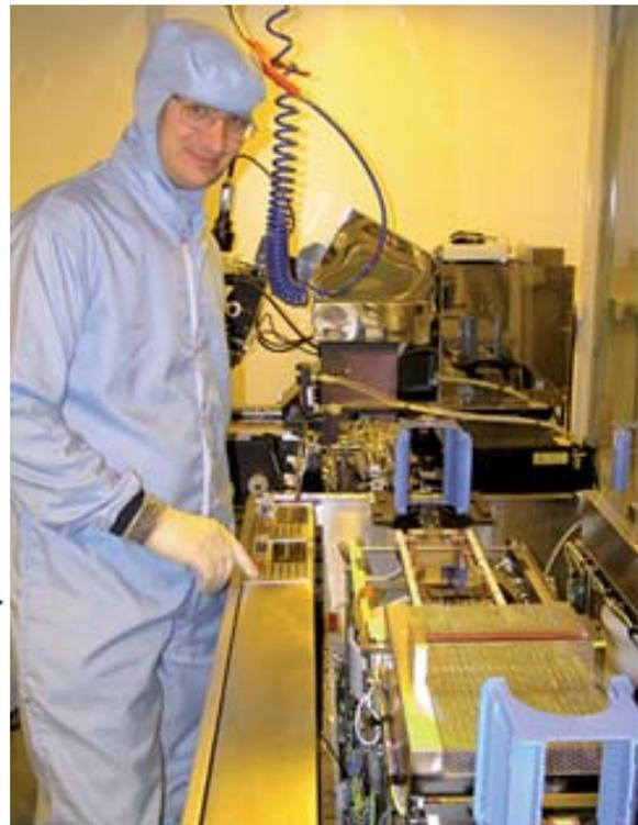
▲ **Figure 2. Track coating and lithography tools for chalcogenide waveguide fabrication.**
