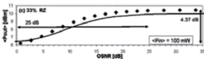
▲ Figure 4b. Measured performance of OSNR for 40 Gb/s RZ signal by measuring average output power from NOLM.
