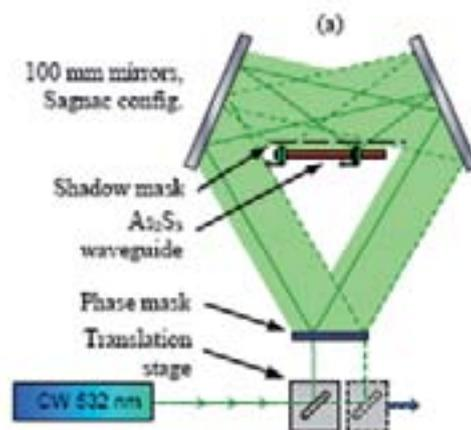
▲ Figure 6. Schematic of custom built scanning Sagnac interferometric system for writing Bragg gratings in waveguides.
