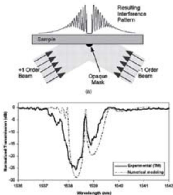
▲ **Figure 7. Mechanism of introducing a defect into a chalcogenide integrated waveguide grating structure to obtain a phase-shifted grating and (b) experimental transmission spectrum (solid curve) of the resulting phase-shifted grating (TM polarization) versus the spectrum obtained from modeling (dashed-dotted curve).**
