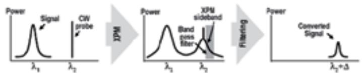
▲ Figure 5a. General principle of all-optical wavelength conversion by using cross phase modulation of signal pulse onto cw probe and then filtering broadened spectrum at desired output wavelength.
