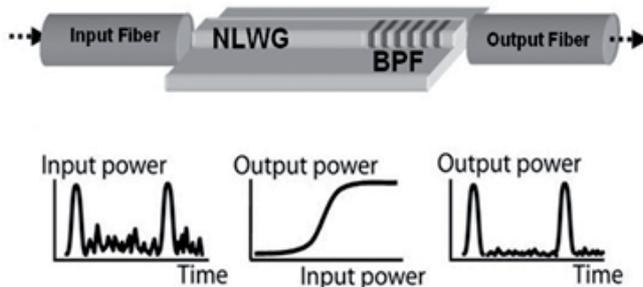
▲ **Figure 1. All-optical signal regenerator concept exploiting optical Kerr effect in nonlinear waveguide (NLWG), which has a bandpass optical filter (BPF) integrated in the same device.**
