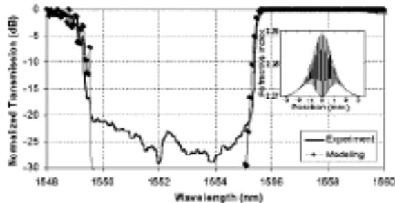
▲ **Figure 3. Experimental and theoretical normalized transmission spectra of a strong grating fabricated in a 5 cm long As<sub>2</sub>S<sub>3</sub> rib waveguide (W=4 μm, H=2.37 μm, h=1.25 μm). Inset: the grating profile used for modeling.**
