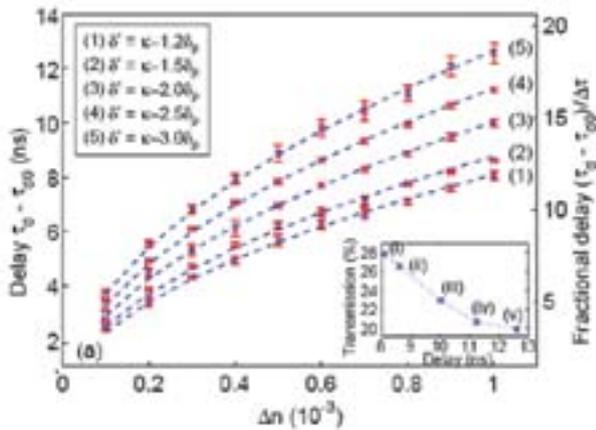
▲ **Figure 2. Calculated delay in nanoseconds (left-hand side) and fractional delay (right-hand side) versus the grating strength for different values of the strain on the fibre. For strong gratings the delay can in principle be well over 10 pulse widths. The inset shows the power transmission versus the strain.**
