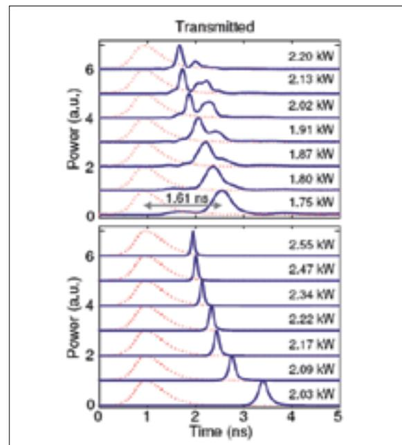
▲ **Figure 1. Measured nonlinear transmission versus input power (top) and associated simulations (bottom). The dotted curve gives the transmission in the absence of the grating. The delay is 1.61 ns at an input power of 1.75 kW, and can be tuned by varying the input power.**
