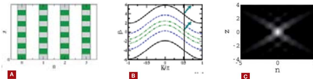
▲ **Figure 4. (a) Waveguide array with phase-shifted Bragg gratings; integer n counts the waveguides; (b) Iso-frequency contours featuring wavelength independent refraction indicated by arrows; (c) Example of a slow light bullet exhibiting nonlinear self-trapping in space and time**
