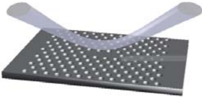
▲ Figure 1. Coupling scheme used: schematic showing the coupling from a tapered fibre to PhC nanocavity
