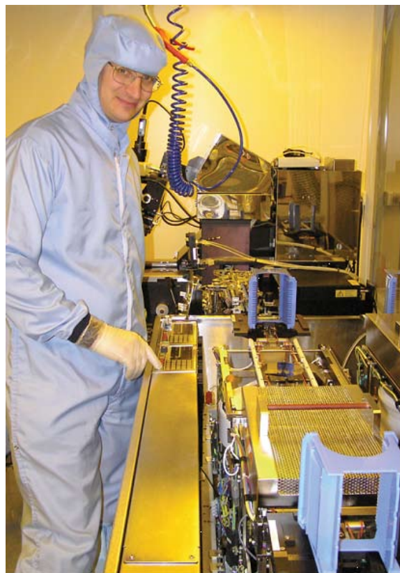
▲ Track coating and lithography tools in the LPC clean room (Steve Madden).
