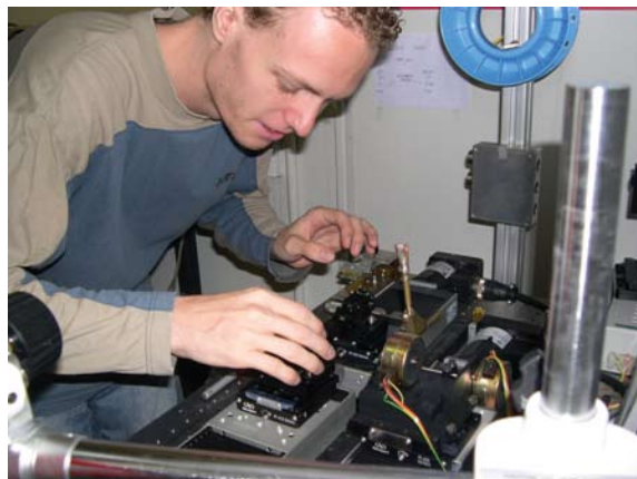
▲ Cameron Smith, Masters student in CUDOS, works on one of the optical fibre taper stations.
