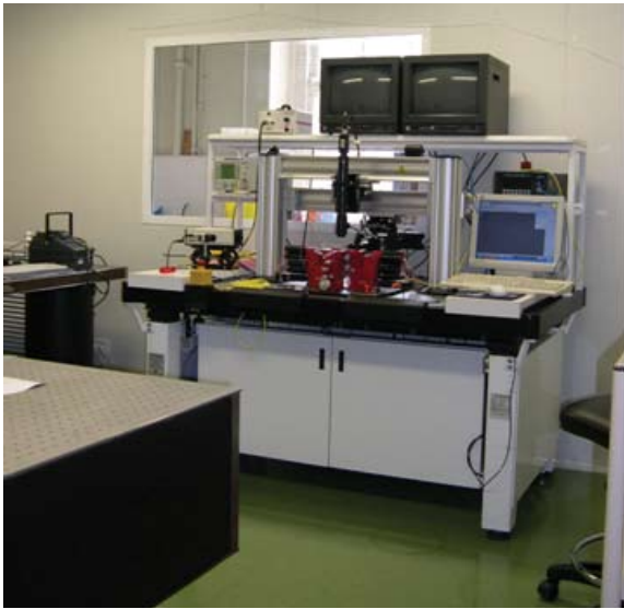
▲ The fibre-waveguide automatic coupling alignment system installed in a Class 350 clean room within the laboratories at CUDOS, University of Sydney.
