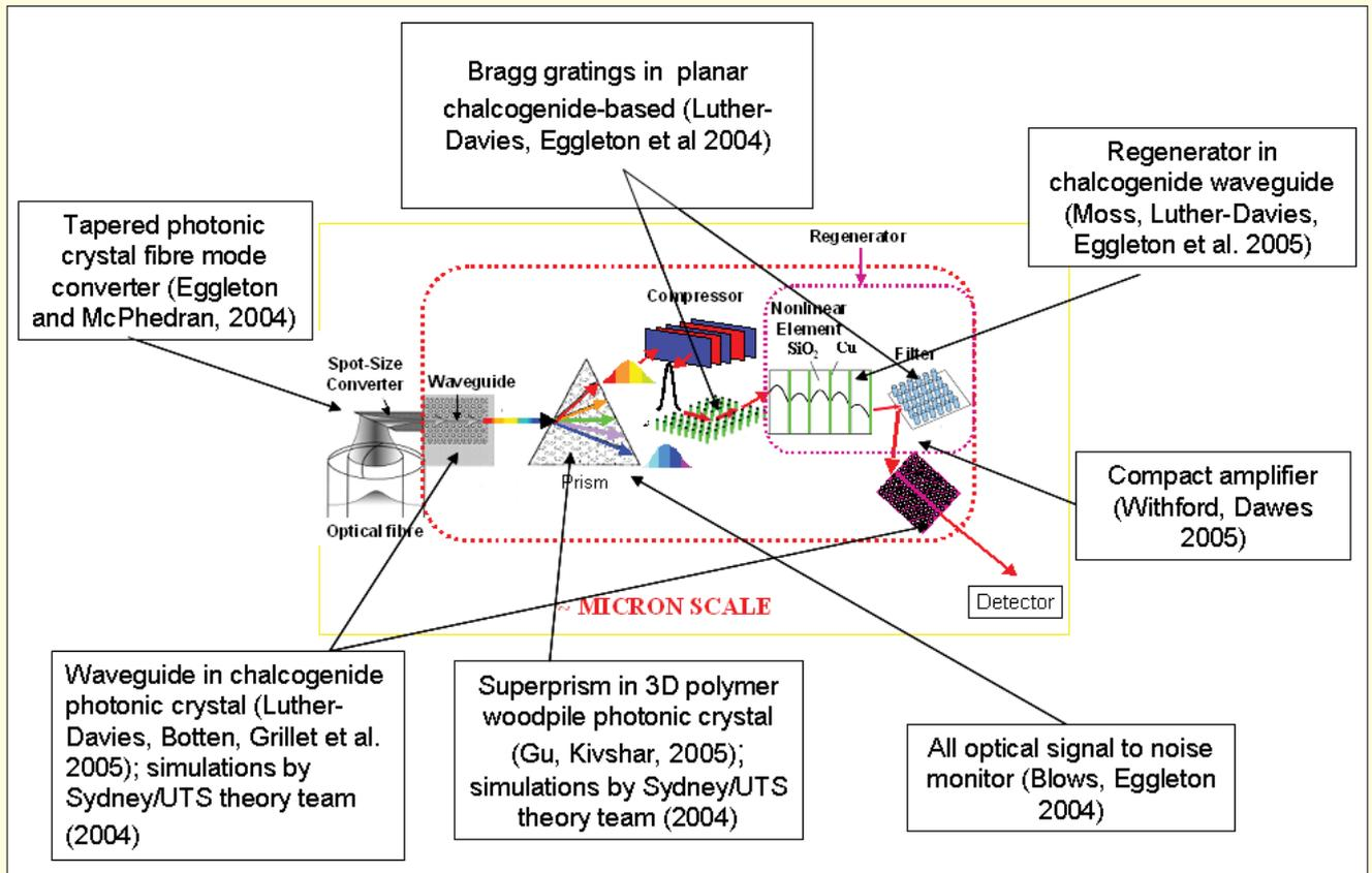
▲ The CUDOS program to date has focused on demonstrating individual functionalities that ultimately would appear in a photonic integrated circuit. Those demonstrated include efficient conversion from single-mode fiber, waveguides and microcavities in photonic crystals, demultiplexing and beam steering using photonic crystals, dispersion control and optical filtering using Bragg gratings, optical performance monitoring and all-optical regeneration and optical amplification.
