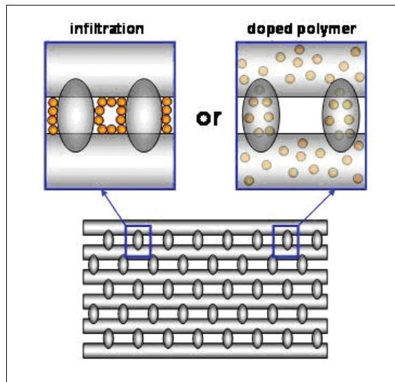
▲ Methods for incorporation of quantum dots (shown in yellow): infiltration and doping.
