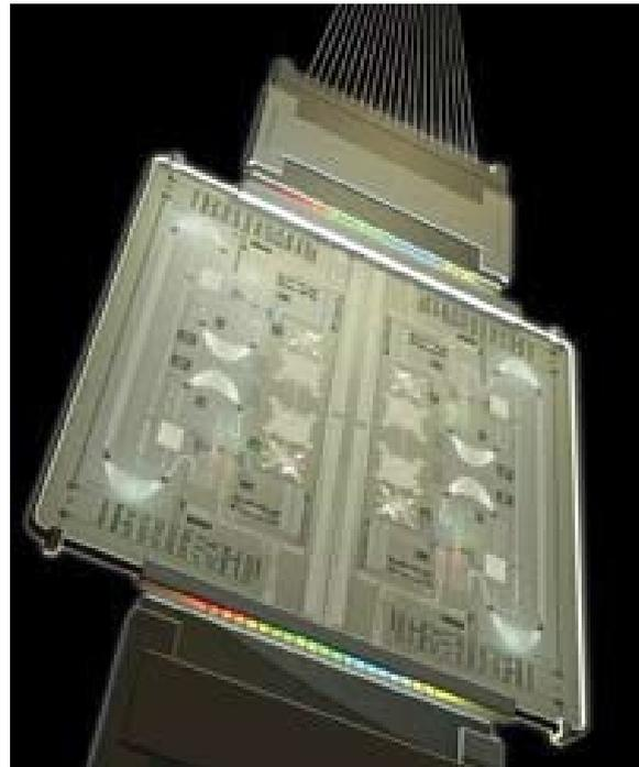
▲ A PIC would look little different to an electronic integrated circuit, except that signals are coupled in and out along optical fibres (from [www.esa.int/SPECIALS/ GSP/ SEM6AE03E4E\\_2.html](http://www.esa.int/SPECIALS/GSP/SEM6AE03E4E_2.html)).
