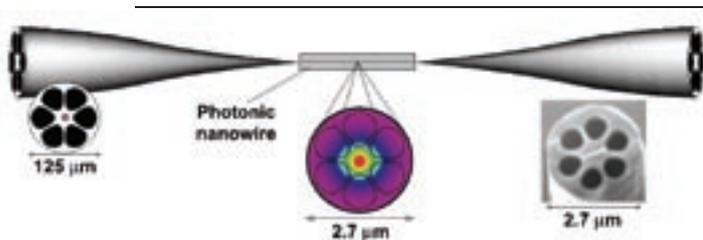
▲ Efficient coupling into nanowires: the mode in a grapefruit fibre is adiabatically coupled into a section where the mode field diameter is less than 1 μm.
