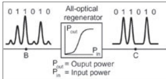
▲ Research in all-optical regeneration, by Mok et al., have shown that regenerators can recover severely corrupted data.
