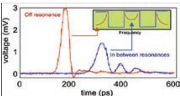
▲ Pulse delay measurement, showing slowing of light near the edge of the photonic bandgap.
