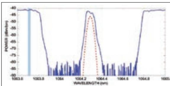
▲ Measured transmission spectrum of the Moiré fibre Bragg grating compared to the input pulse spectrum.
