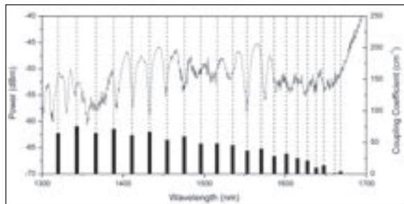
▲ Optical Transmission spectrum from surface waveguide grating in SOI waveguide fabricated by focused ion beam milling (FIB), along with theoretical calculations of the grating peak wavelengths and strengths.
