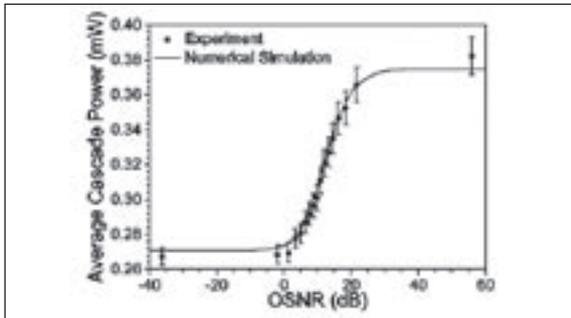
▲ Nonlinear interactions in optical fibre demonstrate strong correlation with OSNR in real time, and will be useful in monitoring future ultrafast networks.
