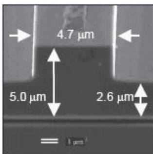
◀ Cross section SEM of an SOI rib waveguide used for fabricating waveguide gratings.
