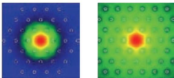
▲ Power distribution of the fundamental mode in MOFs of finite (left) and infinite (right) cross-sections, at the same wavelength in the extended mode region. In the finite case, the mode is confined by the holey region's external boundary but is extremely lossy. In the infinite case the mode is lossless, but spreads far into the cladding.
