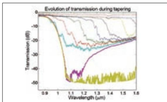
▲ Graph showing shift of transmission spectrum to shorter wavelengths as fibre is tapered.
