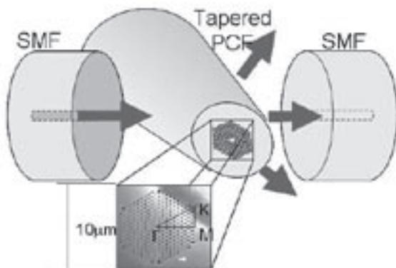
▲ Basic transverse probing geometry.
