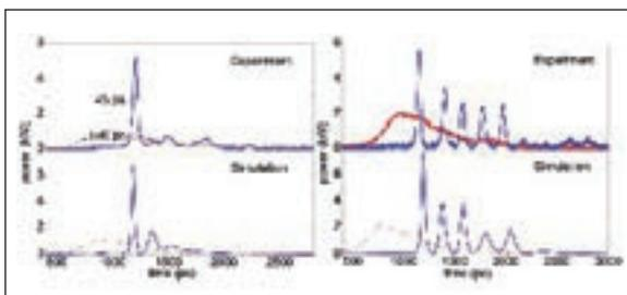
▲ (Left) Pulse compression in a bragg grating and (Right) Pulse train generation via modulational instability.
