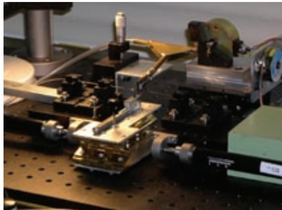
▲ Fibre taper rig with flame brushing in progress.
