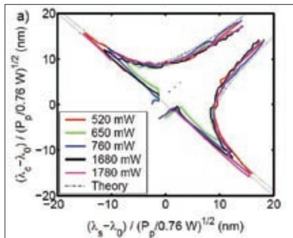
▲ Experimentally obtained contour plots of equal conversion efficiency for the parametric wavelength converter investigated by McKerracker et al. Up to 24 nm of bandwidth has been obtained, and the agreement with theory is excellent.
