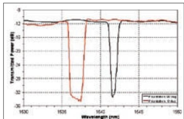
▲ Transmission spectra for photosensitive gratings written in chalcogenide waveguides. The two curves are for two orthogonal polarisations. The grating strength of 22 dB is limited by measurement.
